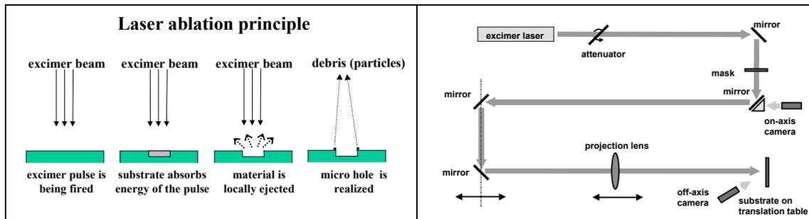
Figure 1: principle of laser ablation.
