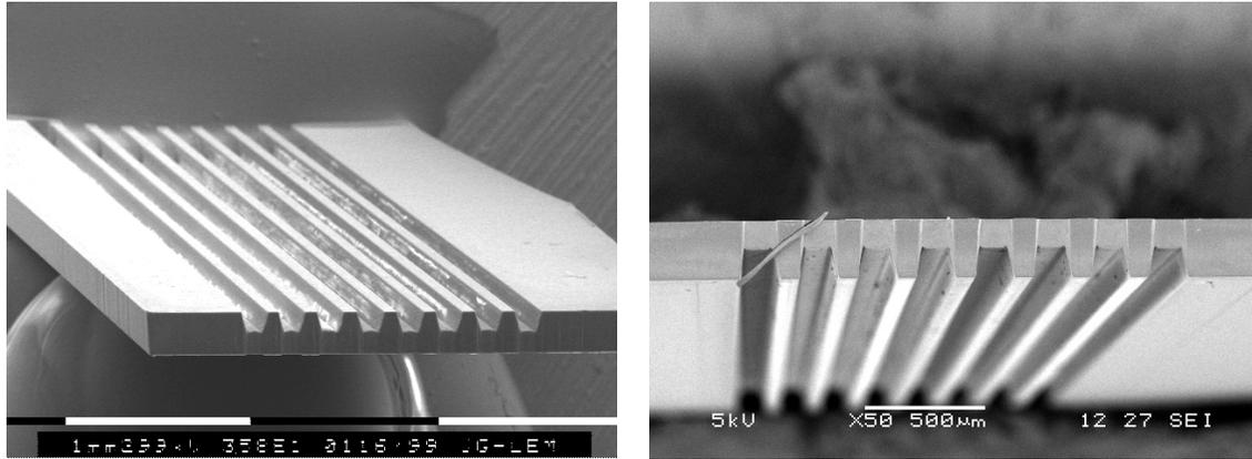
Figure 3: array fabricated with moving aperture method in PC at 248 nm (left), array with mask method in PMMA at 193 nm.
