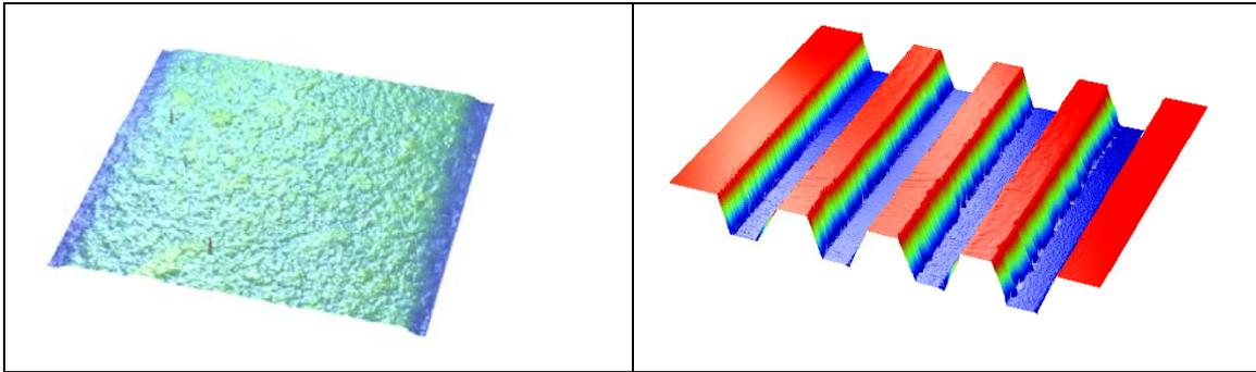
figure 4: surface scan (WYKO) of the groove bottom (left) and a part of the array (right) in PMMA.
