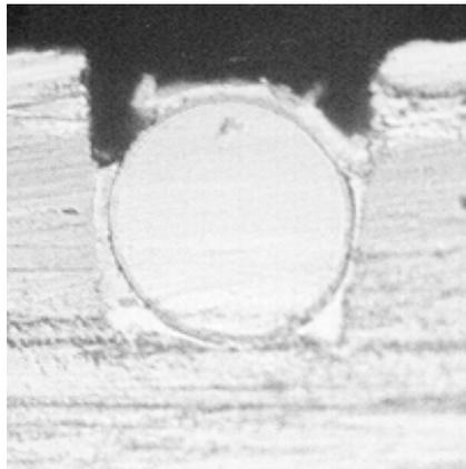
Figure 5: plastic optical fibres fixated in the grooves.
