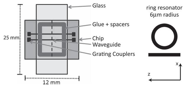
Fig. 3. Schematic top view of a device consisting of a SOI substrate with LC cladding, sealed off by a glassplate with a transparent ITO electrode and polyimide alignment layer (left). Schematic top view of a single ring resonator with the straight waveguide below (right).
