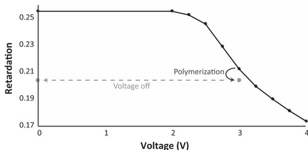
Fig. 1. Retardation of the PLC cell as a function of voltage at a wavelength of 750 nm. Upon polymerization the material is frozen.
