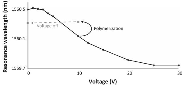
Fig. 6. Resonance wavelength as a function of voltage. The effect of polymerization is shown.
