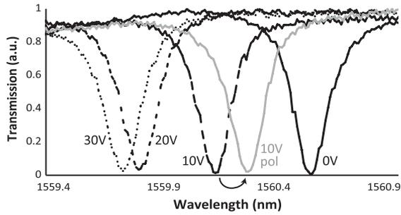
Fig. 5. Transmission of a ring resonator clad with PLC as a function of voltage. Polymerized material results in the gray curve.
