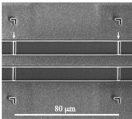
Figure 2. The apparent overlap after stitching is found almost entirely to the right of the stitch line (white arrows), indicating that the edge rate is faster near the edge of the previous rectangle.
