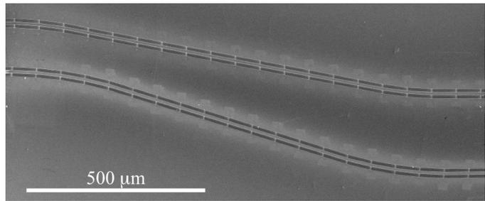
Figure 3. The stitching procedure was used to create smooth bends.
