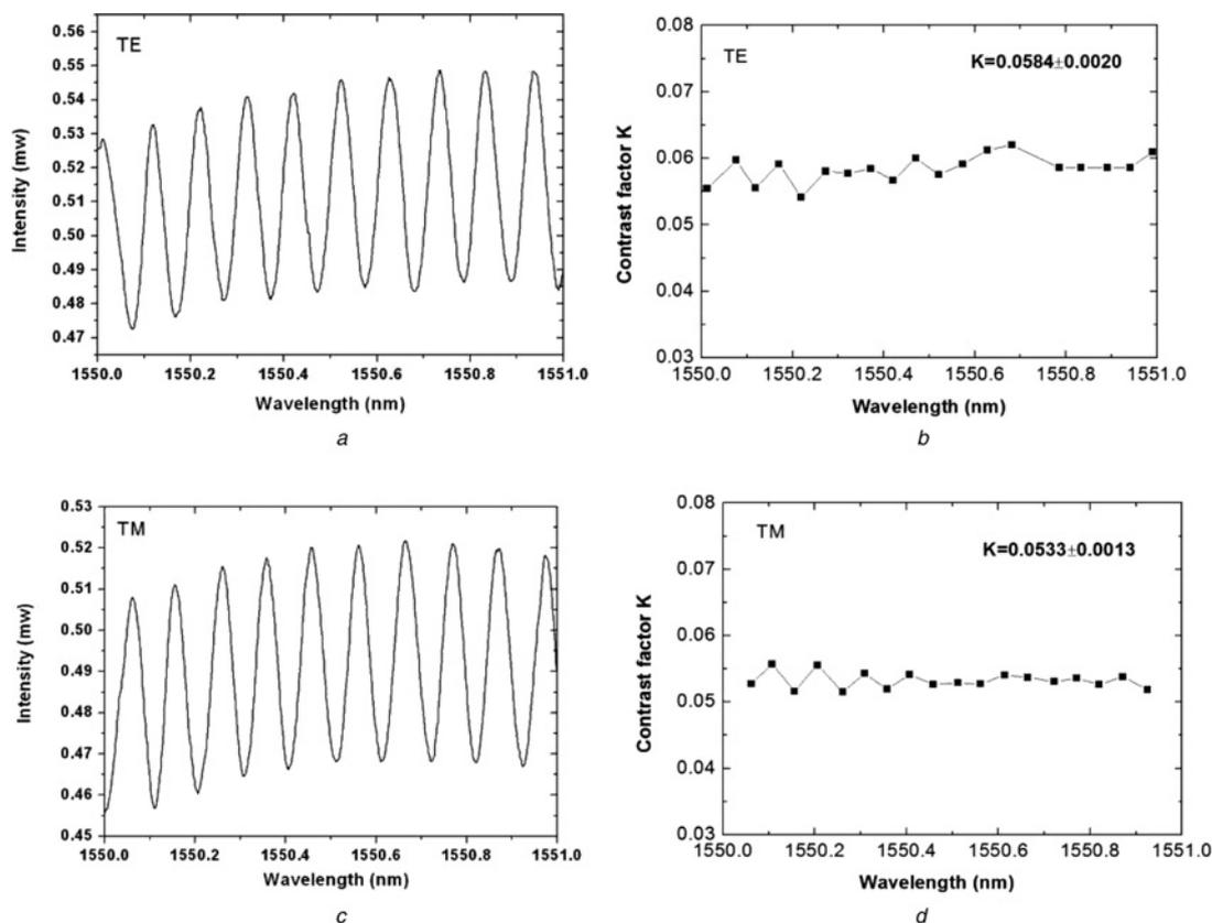
**Fig. 2** Measured Fabry–Perot resonance spectrum for polymer PSQ-L straight waveguides
