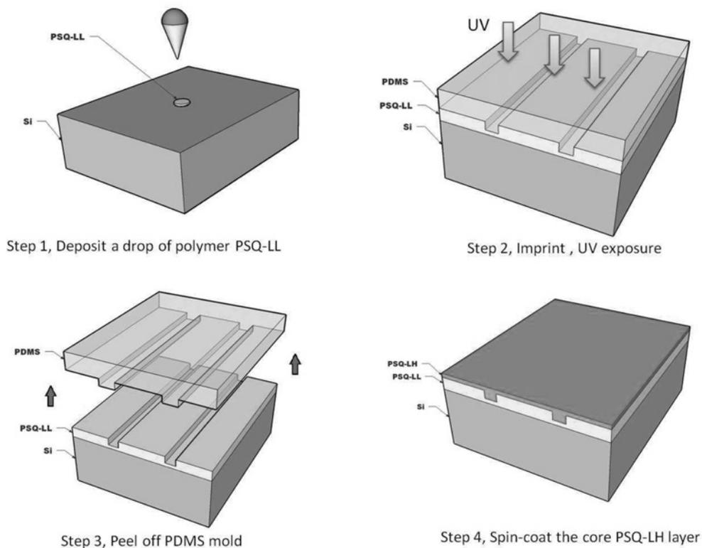
Fig. 1 Fabrication process for polymer PSQ-L waveguides
