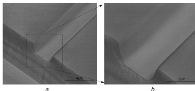
**Fig. 5** SEM pictures of the imprinted waveguide trench
