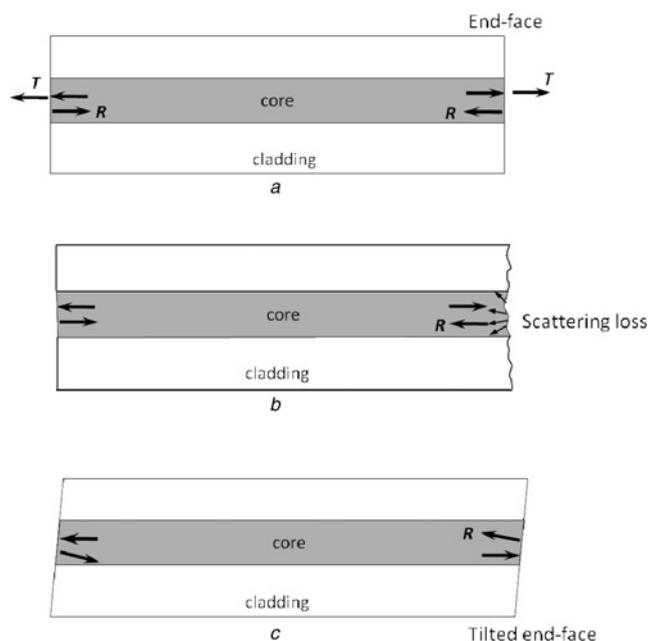
**Fig. 3** Fabry-Perot resonator formed by cleaved waveguides
