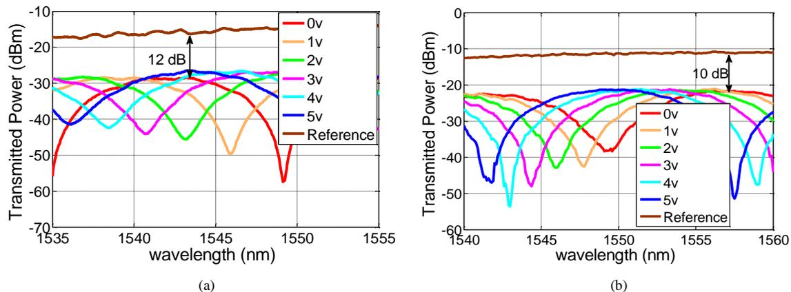
Fig. 2. Transmission spectrums at different bias voltages of two different doping patterns: (a) interdigitated PN junction (b) lateral PN junction
