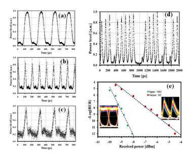
Fig. 2. (a) Input optical data 1010...., (b) Optical clock, (c) Output optical data, (d) PRBS2<sup>7</sup>-1 data output (e) System performance
