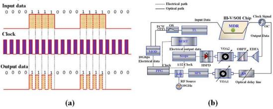
Fig. 1. (a) Illustration of format conversion from NRZ to RZ and (b) Schematic of the experimental set-up used for the format conversion.
