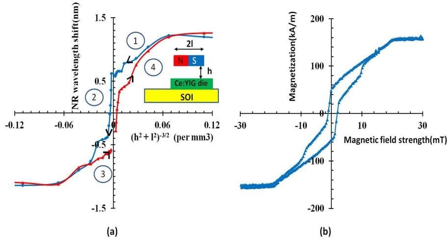
Fig. 11. (a) Nonreciprocal wavelength shift as a function of  $(h^2 + l^2)^{-3/2}$ , where  $h$  is the distance between the magnet and the Ce:YIG layer and  $2l$  is the distance between the two poles of the magnet stack. Negative values for  $(h^2 + l^2)^{-3/2}$  indicate that the magnet was rotated 180 degrees. (b) magnetization curve of the Ce:YIG layer after subtracting the contribution from the paramagnetic SGGG substrate.
