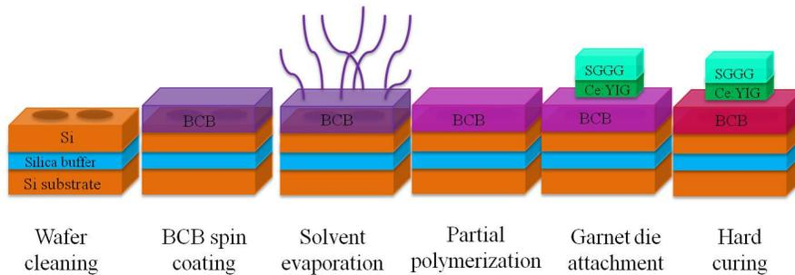
Fig. 6. Schematic illustration of the bonding procedure.
