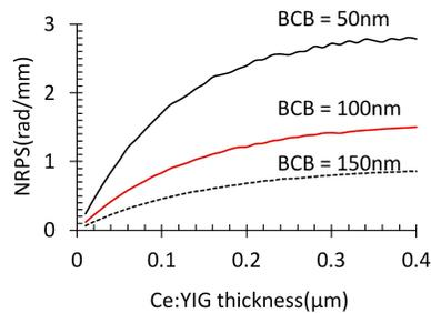
Fig. 5. Nonreciprocal phase shift as a function of Ce:YIG layer thickness for a  $220\text{nm}$  thick silicon waveguide layer thickness and different DVS-BCB bonding layer thicknesses.
