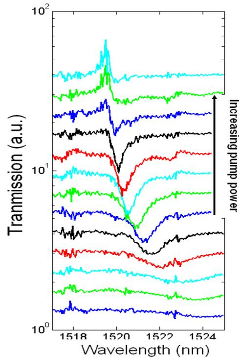
Figure 3. Typical transmission curves for different pump values
