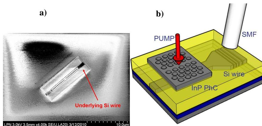
Figure 1. Saturated SEM image showing the Si wire beneath the III-V cavity and schematic of cavity aligned to wire.
