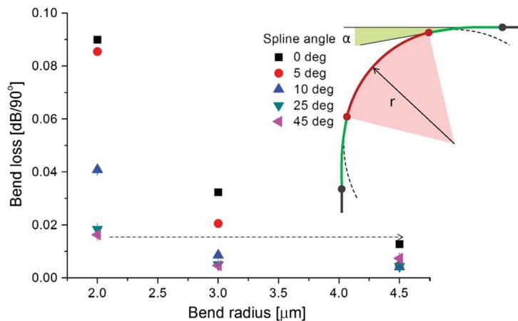
Fig. 7. Bend loss of photonic wires (460 nm  $\times$  220 nm) with 2–4.5  $\mu\text{m}$  bend radius for different spline angles.
