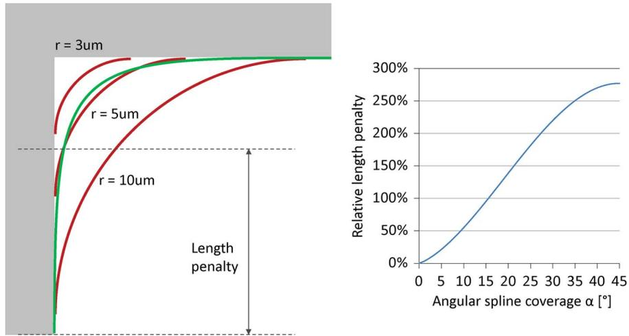
Fig. 3. Bend side length penalty for different angular coverage of the spline section. (Left) Spline bend with  $3\mu\text{m}$  minimum radius, compared with circular bends of 3, 5, and  $10\mu\text{m}$  radius. (Right) Relative length penalty as function of spline angle coverage.
