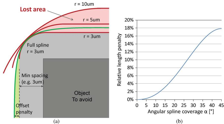
Fig. 4. Bend offset penalty for different angular coverage of the spline section. (a) Spline bend with  $3 \mu\text{m}$  minimum radius compared with circular bends of 3, 5 and  $10 \mu\text{m}$  radius. (b) Relative offset penalty as function of spline angle coverage.
