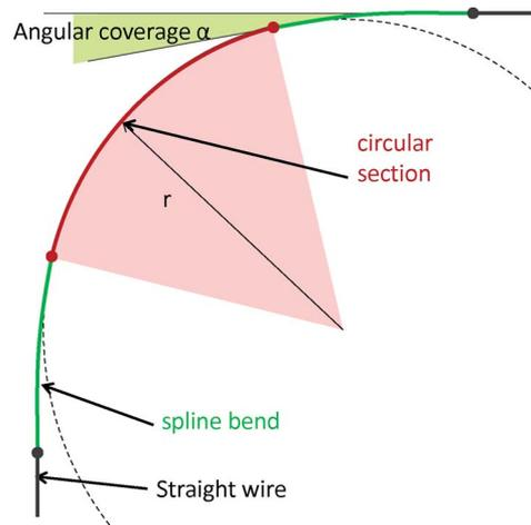
Fig. 1. Bend design using a spline transition between the straight section and the bend section. The curvature is matched at both ends of the spline, which covers an angle  $\alpha$  of the entire bend.
