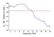
Fig. 2 Small signal frequency response for microdisc laser
