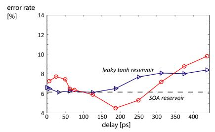
Figure 4. Result of a network of SOAs and leaky tanh reservoirs ( $\eta = 0.1$ ) on a isolated digit speech recognition task. For both kinds of reservoir the interconnection delay is varied and the swirl topology used.
