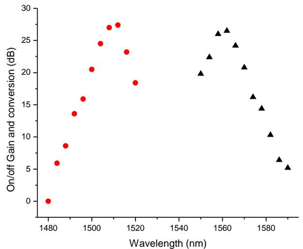
Figure 3: The on/off gain (triangles) and conversion (dots) in function of the probe wavelength.
