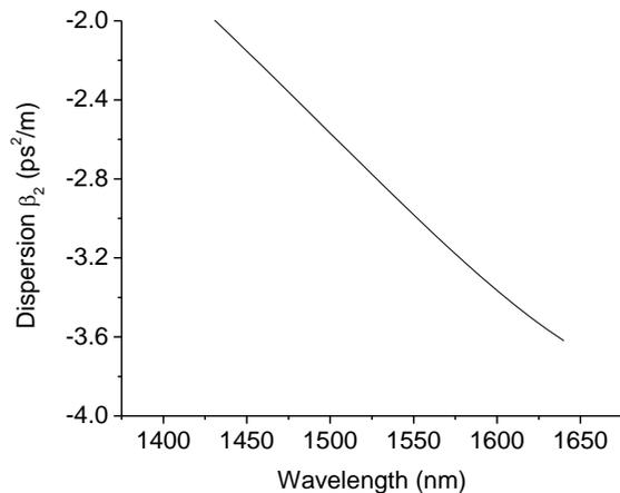
Figure 1: The simulated dispersion of the TE mode of the a-Si:H waveguide used as a function of the wavelength
