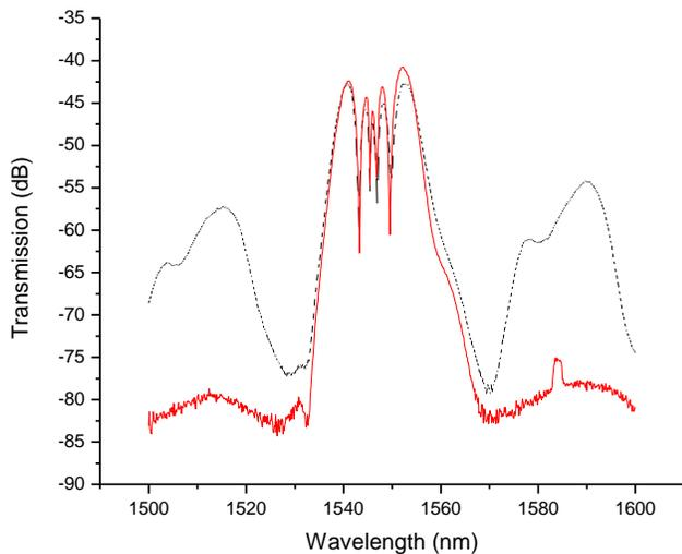
Figure 2: The spectrum at the output of the waveguide when the pulses are not overlapping in time (red, straight) and when they are overlapping in time (black, dotted)
