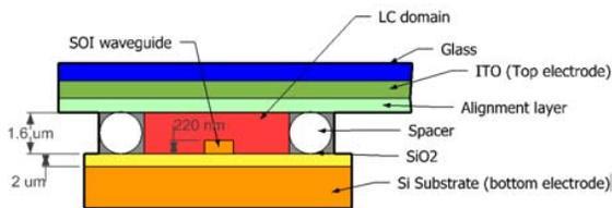
Fig. 1: Cross section diagram of LC-Cell.
