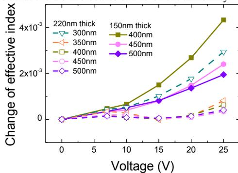
Fig. 3: The calculated change of effective index as a function of voltage depending on width of waveguide with 150 nm (open symbols, broken lines) and 220 nm (solid symbols, continuous lines) thickness. The waveguide dimensions shown here are based on coupling loss considerations.
