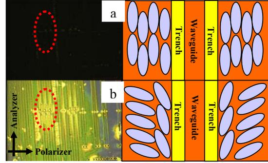
Fig. 4: Polarizing microscope image (left) with top view diagram (right) shows the director orientation on the edges of the trenches. a) at 0 V, b) at 10 V.
