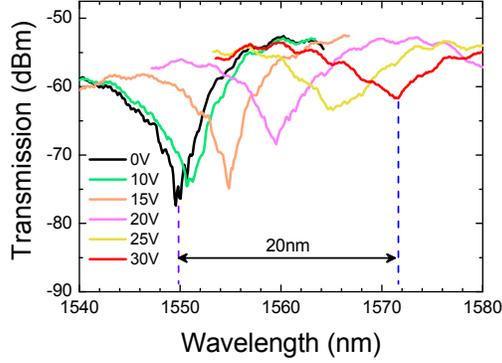
Fig. 2: Transmission spectra of MZI (400 nm width 150 nm thickness), showing a tunability of  $\sim 20$  nm.
