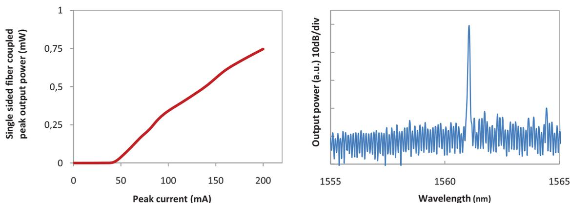
Fig. 2. (a) Fiber coupled laser power as a function of drive current (L-I curve) under pulsed operation at  $20^{\circ}\text{C}$ . (b) Optical spectrum of the laser driven at 55mA
