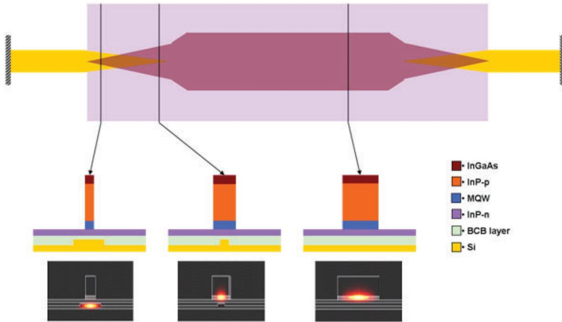
Fig. 1 Top view, cross sections and calculated mode profiles of the III-V/SOI laser
