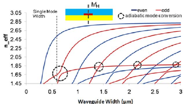
Figure 2. Adiabatic Mode Profile of an asymmetric waveguide.
