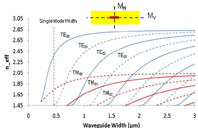
Figure 1. Adiabatic Mode Profile of a symmetric waveguide.
