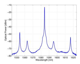
Fig. 3. Optical spectrum of a 7.5- $\mu$ m diameter microdisk.
