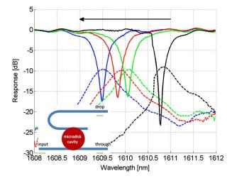
Fig. 10. Schematic layout of the proposed switch (inset) and the influence of the injection current on the through (solid) and drop (dashed) port transmission characteristics of the microdisk cavity [curves for 0, 55  $\mu$ A (0.9 V), 100  $\mu$ A (1 V), and 200  $\mu$ A (1.1 V)].
