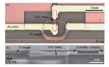
Fig. 21. (a) Top view and (b) cross-sectional view of a fully fabricated resonant detector.
