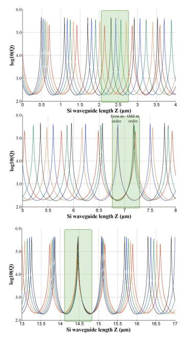
Fig. 9. *Q* factor variation as function of external loop length for resonant modes of a 4  $\mu$ m radius and 0.55- $\mu$ m-thick microdisk coupled to a 200 × 500 nm Si waveguide. Differently colored curves corresponds to the TE(0,31,0) = 1645 nm up to the TE(0,35,0) = 1490 nm resonances of the resonator. The minimum value of *Q* can be arbitrary low and is determined by the coupling rate.
