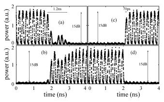
Fig. 11. Switching characteristics of the microdisk electrooptical switch. (a) and (c) are the off and on transients at the through port, respectively. (b) and (d) are the on and off transients at the drop port, respectively
