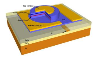
Fig. 1. Schematic representation of a MDL heterogeneously integrated on SOI.
