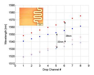
Fig. 19. Experimentally measured channel wavelengths for two 8-channel add-drop multiplexers with 29 nm (circles) and 22 nm (squares) FSR, respectively. The inset shows a microscope image of the fabricated heater with underlying ring resonator.
