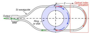
Fig. 8. Microdisk coupled to an outer loop, with a single optical output.
