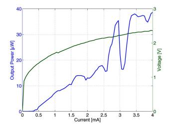
Fig. 2. Output power and voltage vs. current for a 7.5- $\mu$ m diameter MDL.
