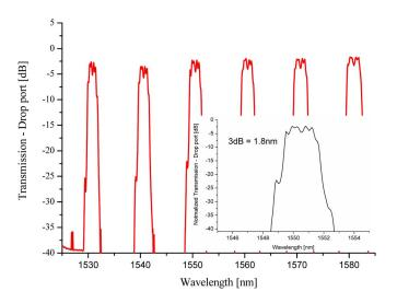
Fig. 17. Spectral response of a tenth order CCF, inset shows details of a single wavelength band.
