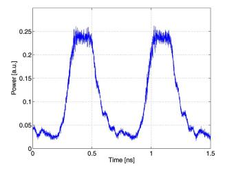
Fig. 5. Direct current modulation response of a 7.5-µm diameter MDL with an electrical driving signal of a periodic square-wave at 1.5 GHz [36].
