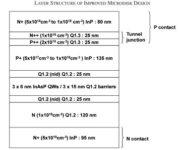
Note: Structure is grown upside down for compatibility with bonding process.
