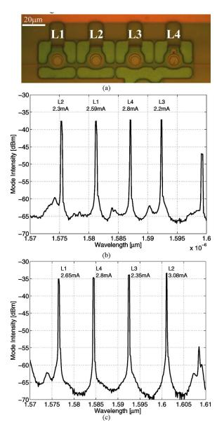
Fig. 4. (a) Fabricated MWL before metallization, composed of four MDLs on a single silicon bus waveguide. (b) and (c) Spectra of MWLs with 6 and 8 nm channel spacing. The bias current of each MDL and the laser number is indicated on the corresponding lasing peak [35].
