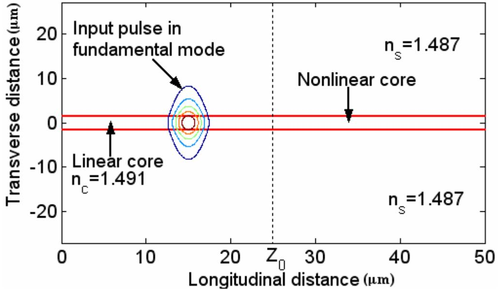
Figure 1. Junction of linear and nonlinear planar waveguides.
