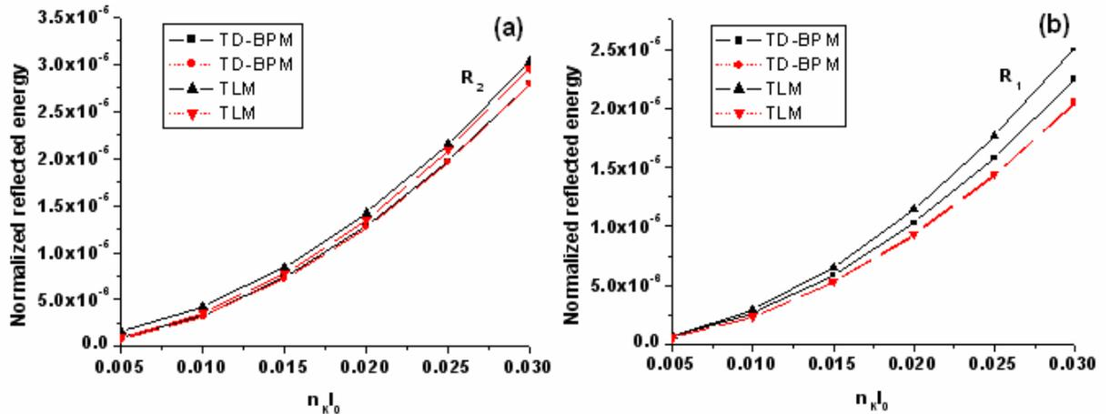
Figure 2. (a) Total reflected energy  $R_2(t)$  and (b) reflected energy in the core  $R_1(t)$ . Pulse durations 18 fs (solid lines) and 36 fs (dashed lines).
