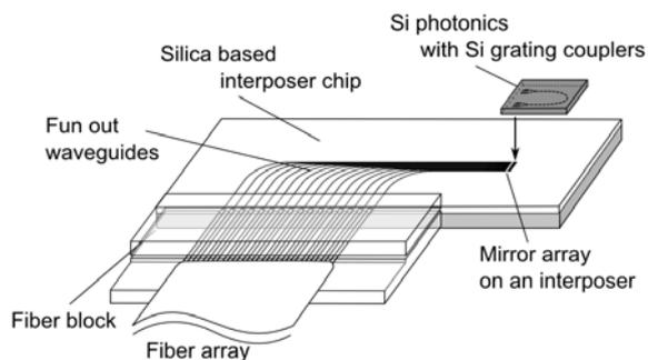
Fig. 1 Schematic of interposer for Si photonics.
