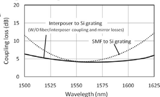
Fig. 2 Predicted coupling loss of interposer.
