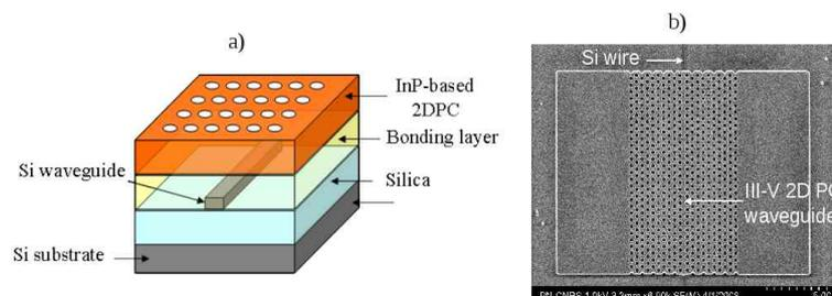
Figure 1. a) Envisaged structure comprising InP PhC layer aligned to the underlying Si waveguide layer . b) Top view of the patterned InP layer, demonstrating the high accuracy alignment.
