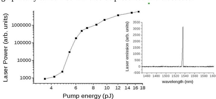
Figure 2. Laser power vs Pump energy log-log scale. Inset:Laser spectrum for pump energy 9.6pJ.
