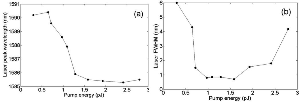
FIG. 5. (a) Peak emission wavelength vs pump energy; (b) FWHM vs pump energy.
