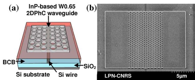
FIG. 1. (Color online) (a) Schematic of the sample. (b) SEM image of the sample.
