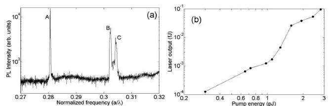
FIG. 4. (a) PL spectrum of the hybrid structure. The three peaks, A, B, and C correspond to the low- $v_g$  modes of Figs. 2(a) and 2(b) Laser emission intensity observed in mode A vs pump pulse energy.
