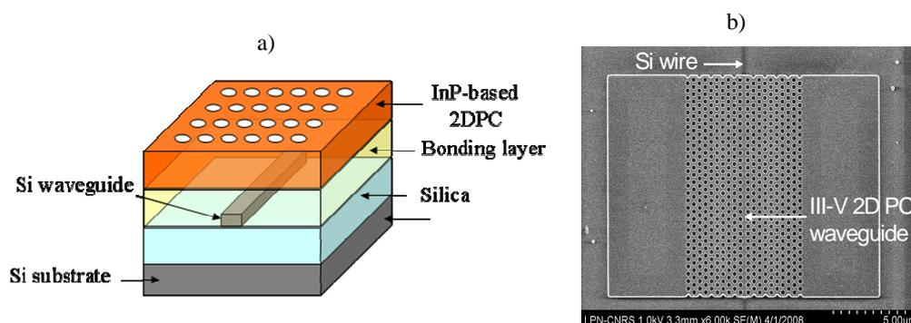
Fig.1. a) Schematics of the hybrid structure. b) SEM image of the 2D PC waveguide aligned to the Si Wire
