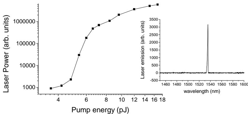
Fig.2. Laser power vs Pump energy in log-log scale. Inset: Laser spectrum for Pump energy = 9.6pJ.
