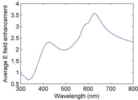
FIG. 7. (Color online) Spectrum of the average  $E$  field enhancement for 8 nm spacing between MNPs (when integrated over in the middle sublayer excluding the MNP area).
