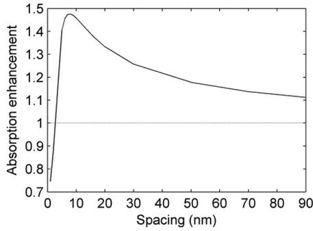
FIG. 4. Absorption enhancement with MNPs in function of particle spacing.
