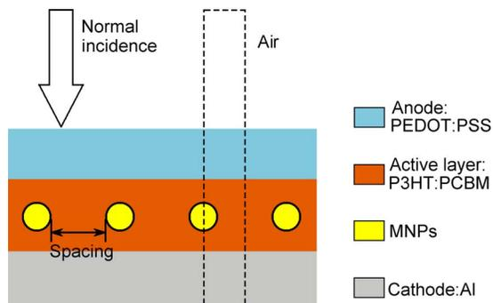
FIG. 1. (Color online) Schematic figure of the model of the solar cell with MNPs. In simulations only the dotted domain is used.
