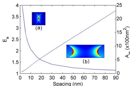
FIG. 5. (Color online) Spacing dependence of average  $E$  field enhancement (solid line) and average mode size (dashed line). The insets show the  $E$  field enhancement at 425 nm with different spacings: (a) 2 nm and (b) 20 nm.
