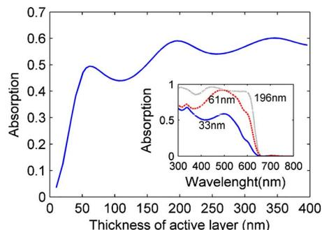
FIG. 3. (Color online) Thickness dependence of absorption in the active layer. The inset shows the absorption spectra for active layers with varying thicknesses.
