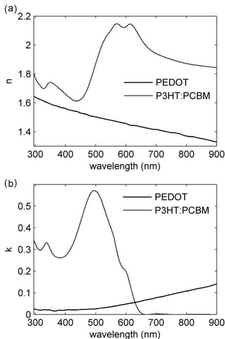
FIG. 2. Real part (a) and imaginary part (b) of refractive indices of PEDOT and P3HT:PCBM (1:1).
