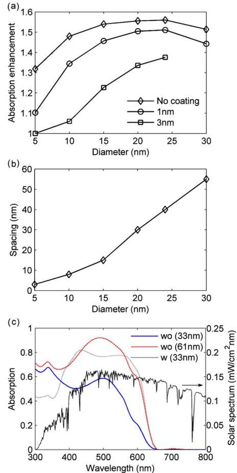
FIG. 8. (Color online) (a) Optimized absorption enhancement as a function of MNP diameter with and without coating. (b) Optimum spacing corresponding to absorption enhancement in (a). (c) Absorption spectra for a solar cell (33 nm) with (w) and without (wo) 24 nm diameter MNPs and for a solar cell (61 nm) without MNPs and AM 1.5G solar spectrum.
