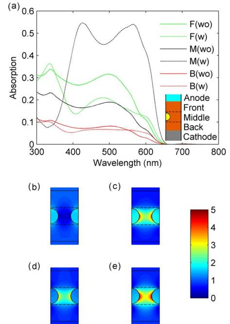
FIG. 6. (Color online) (a) Absorption spectra with (w) and without (wo) MNPs in front (f), middle (m) and back (b) layers with MNPs embedded in the middle layer with 8 nm spacing. Representative figures of electric field enhancement corresponding to 8 nm spacing between MNPs at (b) 330 nm, (c) 425 nm, (d) 485 nm, and (e) 565 nm.
