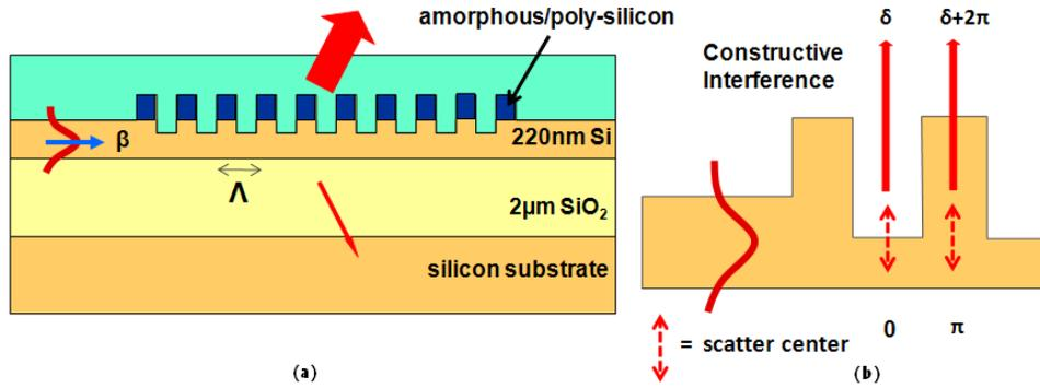
Fig. 1: Cross section of a silicon overlay grating (a) and a schematic illustrating the physical principle of high directionality in these overlay gratings (b).
