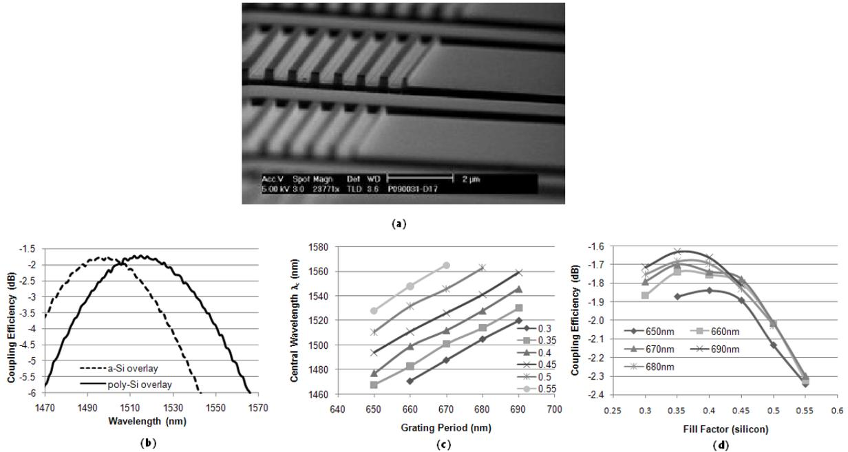
Fig. 2: Side view image of a silicon overlay grating (a). Comparison of the coupling spectrum for an amorphous silicon overlay grating and a polysilicon overlay grating (period=660nm and duty cycle=0.4)(b) Measurement results of a sweep of 1D fiber couplers (a-Si overlay) (c,d).
