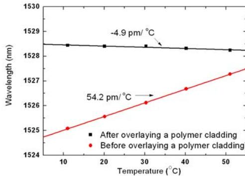
Fig.3 Linear fit of the wavelength versus temperatures
