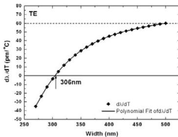
Fig.1 Calculated wavelength temperature dependence of TE mode for SOI waveguide with polymer overlay as a function of waveguide width
