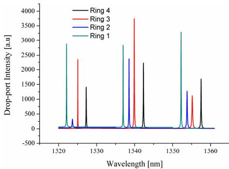
Fig. 2. Drop-port spectrum of 1x4 ring (de)multiplexer.
