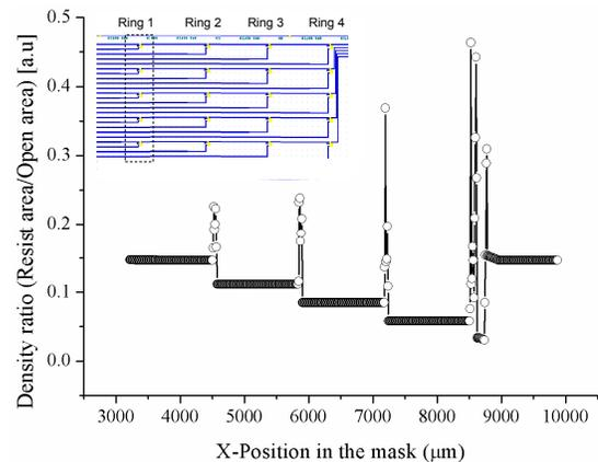
Fig. 1. Loading of different ring resonators. Inset-mask layout showing different rings.
