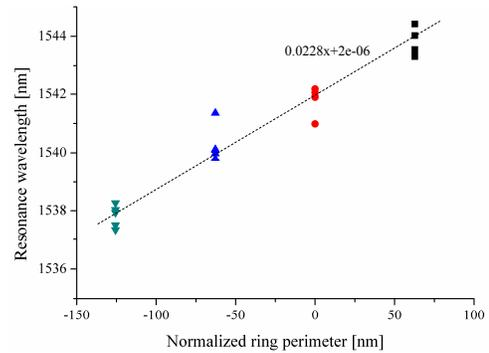
Fig. 4. Resonance wavelength shift as a function of perimeter.
