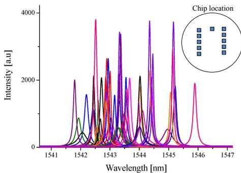
Fig. 3. Drop-port spectrum of 55 ring filters from 11 chips.
