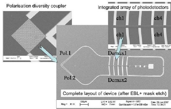
Figure 1: Overview of the polarization diversity demultiplexer receiver, the four channels are separated by the white trenches
