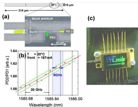
Figure 4: View (a), performance (b), and packaging (c), of a monolithic wavelength-controlled PhC tuneable laser.
