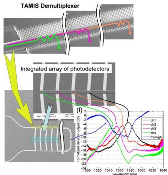
Figure 2 : Zoom on the “TAMIS” demux (top) and spectra showing its performances (bottom, 4 channels, 10 nm spacing), adapted to CWDM
