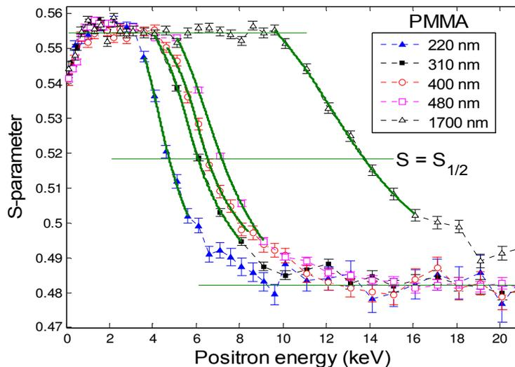
Figure 1. S-parameters as a function of the implantation energy for the poly(methyl-methacrylate) (PMMA) films.
