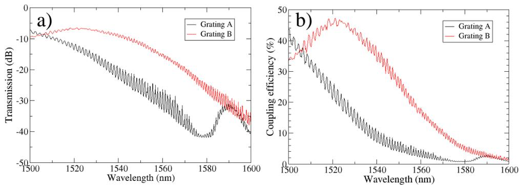
Fig. 2: a – Transmission through a  $50 \mu\text{m}$  wire with two grating couplers, for two different grating;.
