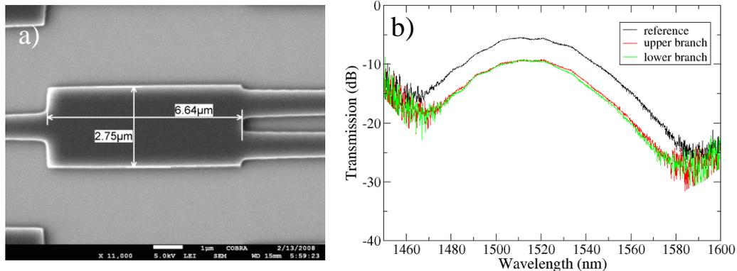
Fig.5 : a – SEM image of a fabricated MMI ;
