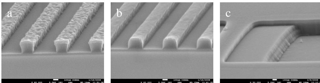
Fig 1: a – Resist pattern of a grating without post-bake;
