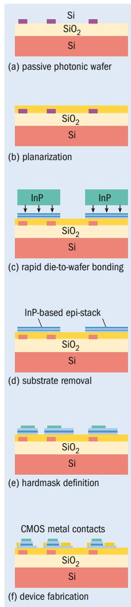
**Fig. 2.** (left) The PICMOS approach to building an InP microlaser coupled to a silicon-wire waveguide involves the fabrication of a passive photonic silicon wafer **(a)**, its planarization **(b)** and the addition of InP die **(c)**. The substrate is then removed from these InP structures **(d)**, before a mask defines the laser **(e)** and CMOS metal contacts are added **(f)**.
