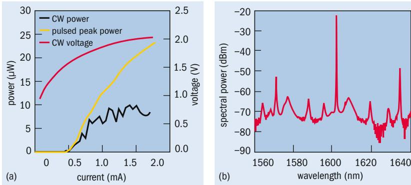
**Fig. 6.** (above) Performance characteristics at 20 °C for a 7.5  $\mu\text{m}$  disk laser **(a)**. The continuous-wave lasing spectrum at 1.4 mA drive current, which has been normalized for the fiber-coupler efficiency and on-chip propagation loss, reveals the dominant lasing wavelength at 1.6  $\mu\text{m}$  **(b)**.
