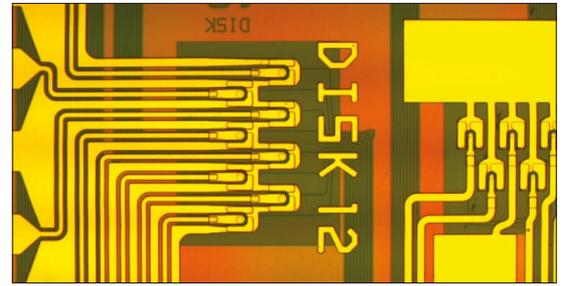
on silicon, employs an efficient die-to-wafer bonding process to transfer small III-V-based epitaxial dies onto SOI wafers. Following substrate removal, the III-V epilayers are then processed using classical wafer-scale processes (see figure 2 for details).
