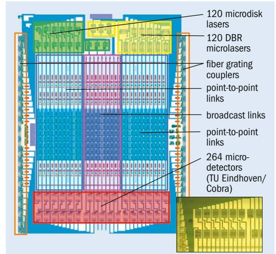
conference, which was held this March in Anaheim, CA, USA. This optical source was formed by etching the microdisk structure in a thin InP-based layer bonded on top of the silicon waveguides (see figures 4 and 5 pxx). The disk supports whispering gallery modes confined to the microdisk's edges, and a top contact can be added in the device's center without introducing additional optical losses.
