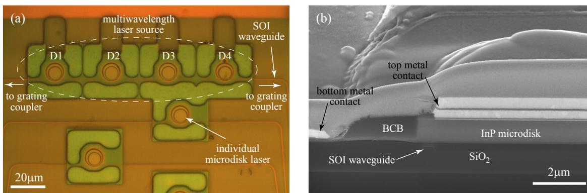
Fig. 1. (a) Top view of the sample (before metallization); (b) FIB cross-sectional picture of a completely fabricated microdisk laser.
