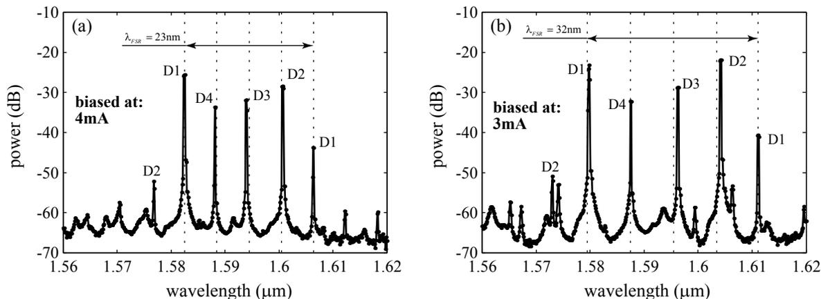
Fig. 3. Normalized spectra of the MWLs from the left end of the bus SOI waveguide when the four microdisk lasers were simultaneously biased at the same current, (a) for 10  $\mu\text{m}$  diameter group and (b) for 7.5  $\mu\text{m}$  diameter group. The dashed lines are separated by  $\lambda_{FSR}/4$ . The corresponding disk number is marked on each of the laser peaks (cf., Fig. 1).
