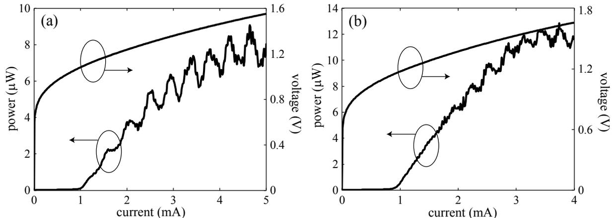
Fig. 2. LIV curves of microdisk lasers with (a)  $10\mu\text{m}$  diameter and (b)  $7.5\mu\text{m}$  diameter under CW. Powers were normalized by the efficiency of the grating coupler.
