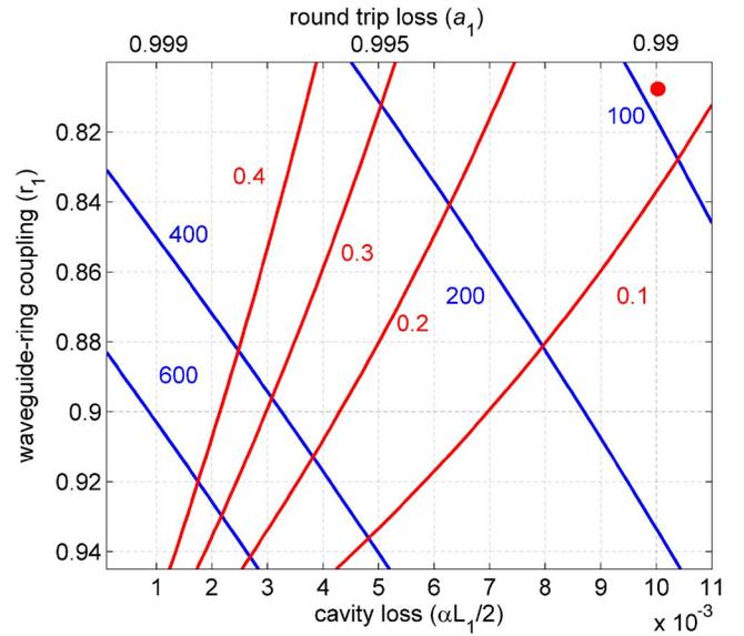
FIG. 5. (Color online) The measured device performance shown on the Finesse- $D_{\text{max}}$  contour for the case  $r_2\sim 0.92$ .
