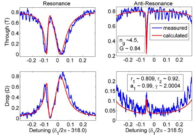
FIG. 3. (Color online) The measured transmission (blue) and the theoretical fit (red) as a function of  $\delta_1$ . Note that the narrow resonance (right) is slightly offset from the antiresonance of  $R1$ .
