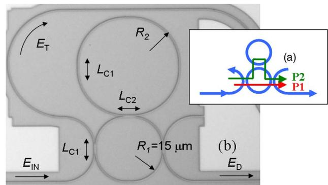
FIG. 1. (Color online) Schematic structure (a) and microscope image of the fabricated device (b) of the two-ring resonator system.  $E_T$  is the E field in the through port, and  $E_D$  that in the drop port.
