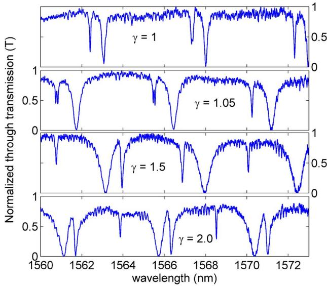
FIG. 2. (Color online) The measured through transmission for various  $\gamma$ . Note the fact that the resonance order is large ( $>300$ ), the Vernier effect is apparent in  $\gamma=1$ , where there are two distinct resonances instead of resonance splitting.
