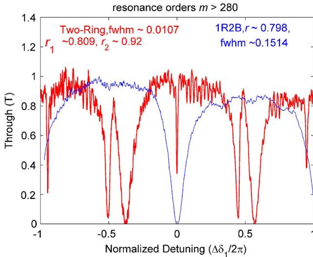
FIG. 4. (Color online) The comparison of two-ring and single-ring transmission spectra as a function of the relative normalized detuning from each resonance.
