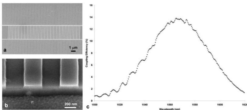
Fig. 2. Fiber grating couplers for SOI waveguides fabricated by a two-step thermal Nanoimprint Lithography (NIL) process. (a) SEM picture of the fabricated grating coupler with a 630 nm period, 50 % filling factor and grating etch depth of 40 nm. (b) Detail of the grating teeth. (c). Experimentally determined fiber-to-waveguide coupling efficiency as a function of wavelength.
