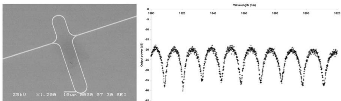
Fig. 1. SOI Mach-Zehnder interferometer fabricated by a single-step thermal Nanoimprint Lithography (NIL) process. (a) SEM-picture. (b) Measured output power as a function of wavelength.
