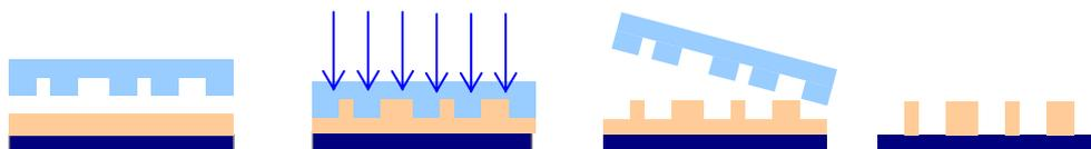
**Figure 1.** Basic steps in UV-NIL: mold and substrate alignment, resist curing, mold release and break-through etch.
