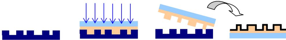
**Figure 3.** Fabrication of transparent molds by nano imprint: imprint in PAK on top of a quartz substrate, deposition of silicon oxide and anti-adhesion treatment.
