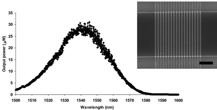
**Fig. 2:** Measurement data of fiber-to-fiber transmission via two gold grating couplers on top of a 10 μm wide SOI waveguide. Input power is set to 1 mW. Inset: SEM-picture of a gold grating coupler prototype. Bar length is 3 μm.
