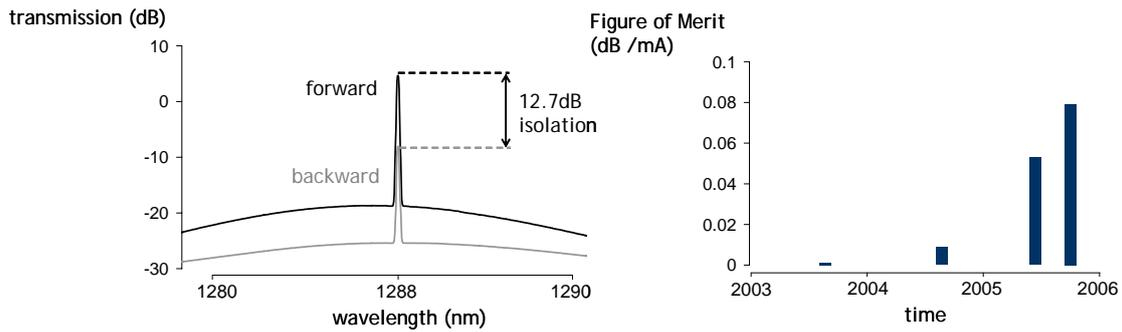
Figure 1: (left) Spectrum of the isolator transmission in both propagation directions, showing 12.7dB optical isolation - (right) Evolution of the demonstrated figure of merit with time.
