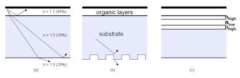
**Figure 1.** (a) Light extraction is limited by total internal reflection. The percentages are an estimation of the amount of light in each layer. (b) The grating at the interface between substrate and air. (c) An RC<sup>2</sup>LED is an OLED fabricated on top of a cavity. The cavity is made from a low refractive index material sandwiched between 2 high refractive index layers.
