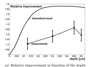
for  $\lambda = 500$  nm, depth = 500 nm, fill factor 50%
