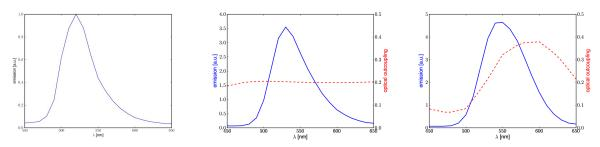
(a) The emission spectrum of the EL (b) Emission and (simulated) optical (c) Emission spectrum and (simlayer of table 4.1. extraction of the reference OLED ulated) optical extraction of the RC<sup>2</sup>LED
