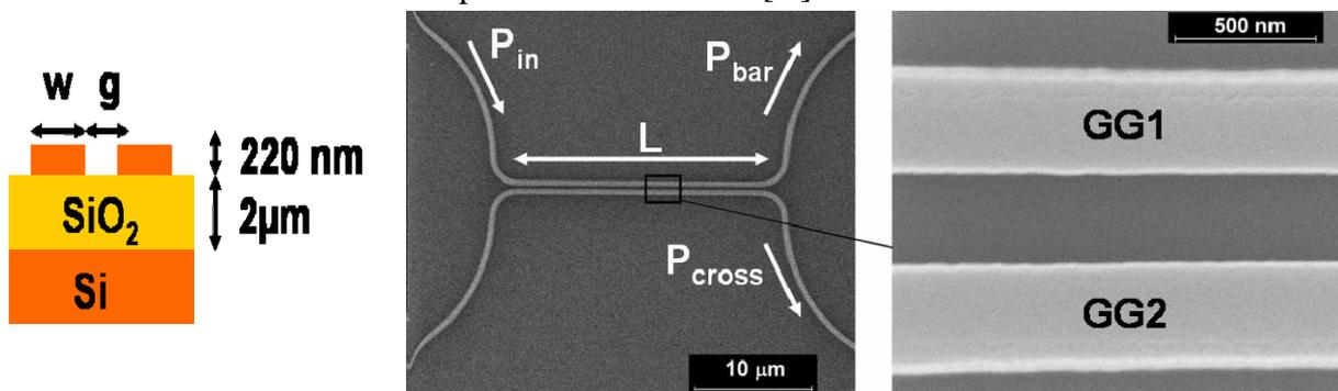
**Figure 2: directional coupler: cross-section (left), SEM-picture + detail (right)**
