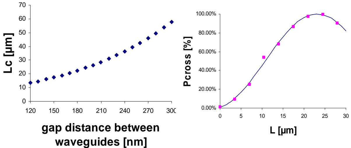
**Figure 3: Simulation of  $L_c$  in function of  $g$  with  $w=400\text{nm}$  at  $\lambda=1.55\mu\text{m}$  (left); Measurement of  $P_{\text{cross}}$  (squares, right) + theoretical fitting (full line, right) at  $\lambda=1.57\mu\text{m}$**
