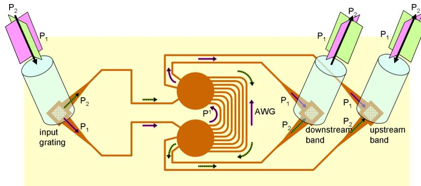
Fig. 3. Principle of a polarization independent duplexer using a polarization splitting grating coupler and bidirectional propagation through an AWG. Both fiber polarizations  $P_1$  and  $P_2$  travel through the same set of grating arms in opposite direction. At the output the polarizations can be recombined again with 2-D grating couplers.
