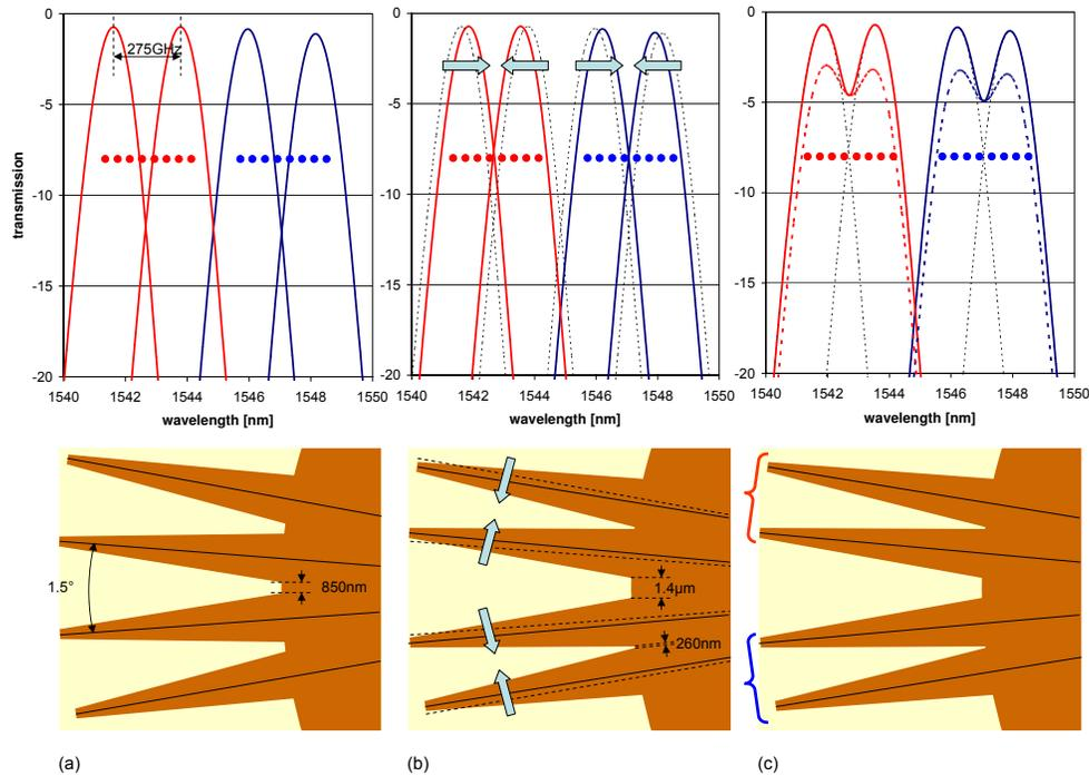
Fig. 4. Design of the AWG. (a) The transmission of the AWG output ports when located at their original channel spacings of  $275\text{ GHz}$ . (b) The output ports are shifted towards each other in pairs. (c) When the signals in the ports are added up, two broad wavelength bands form. Full line: signals combined electrically (power); dashed line: signals combined using a lossless symmetric Y-junction.
