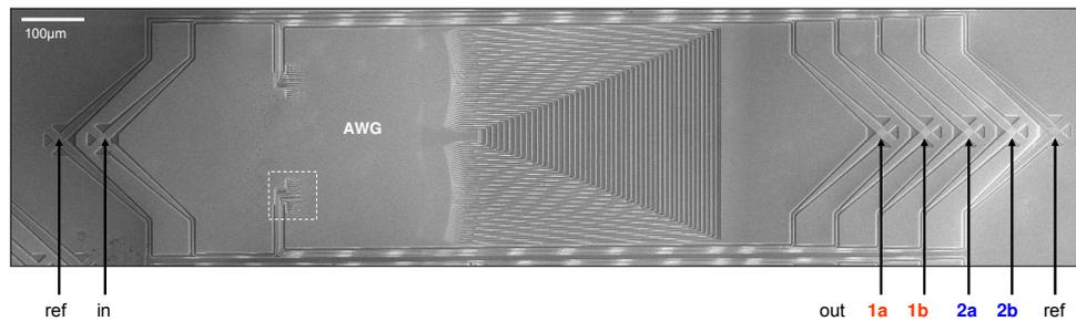
Fig. 6. SEM of fabricated duplexer. The outermost fiber couplers are directly connected and are used for as alignment and reference. The AWG has a  $600 \times 350 \mu\text{m}^2$  footprint. The two outputs for each wavelength band are not grouped but characterized individually.
