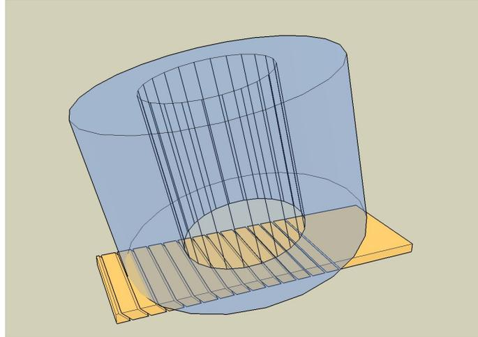
Figure 1: Schematic drawing of the slanted fiber coupler.
