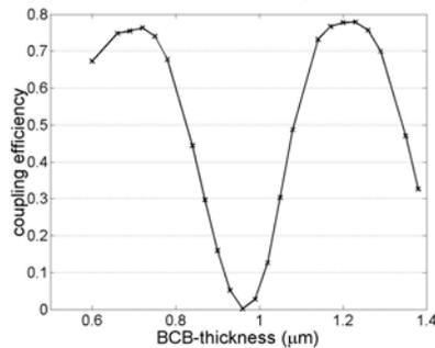
Fig. 3. Maximum coupling efficiency as a function of BCB-thickness.
