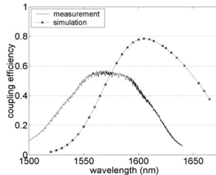
Fig.5. Measured and simulated coupling efficiency.
