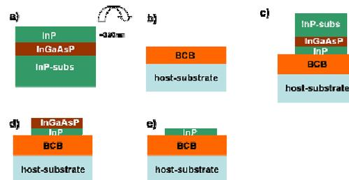
Fig.2. BCB-bonding procedure.
