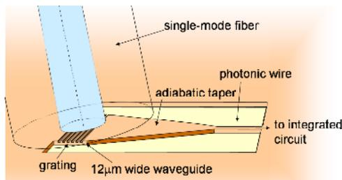
Fig. 1. Coupling principle for out-of-plane coupling between single-mode fiber and photonic wires.
