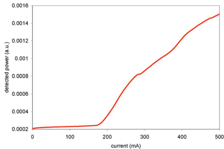
Figure 7. Power – current characteristic of the bonded laser diode. Light is collected from the SOI waveguide using a lensed fiber.
