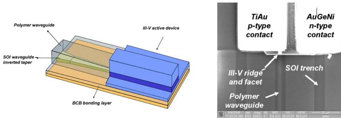
Figure 6. Bonded photodetector structure based on an inverted taper structure. Top view of fabricated structure. The inverted SOI taper is not visible as it is buried underneath the polymer waveguide.
