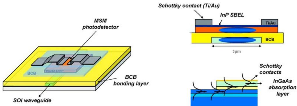
Figure 4. Metal-Semiconductor-Metal photodetector coupling structure
