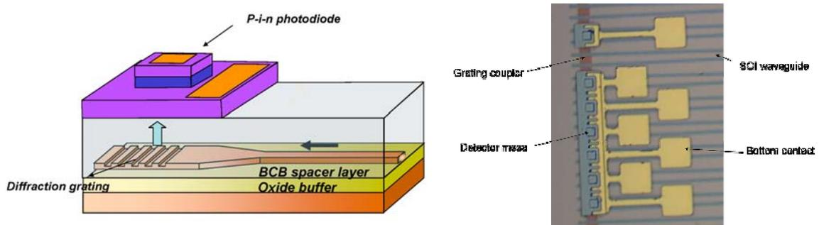
Figure 1. Coupling structure of a bonded surface illuminated photodetector and a top view picture of fabricated structures
