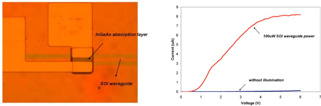
Figure 5. Fabricated devices and measured current versus voltage characteristic with and without illumination.
