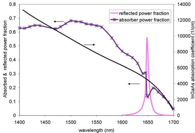
Figure 3. Simulation of the absorbed and reflected power fraction versus wavelength
