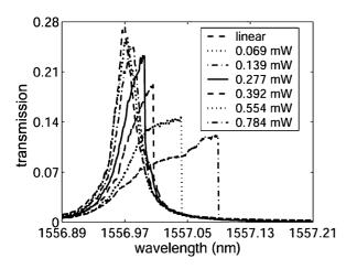
Fig. 15. Normalized transmission of the drop port for different input powers. The linear pass and drop transmissions are indicated as reference. Bistability is obtained for powers equal and above 277 μW.
