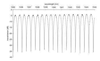
Fig. 4. Normalized transmission of a  $1 \times 1$  MZI with a 1 mm delay length in one arm
