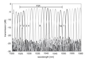
Fig. 6. Overlayed transmission spectra of a 16-channel AWG with 200 GHz channel spacing. The transmission is normalized to give the transmission of the actual AWG.
