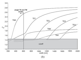
Fig. 1. Dispersion diagrams for a wires at 1550 nm wavelength: (a) oxide cladding and (b) oxide bottom and air topeladding.
