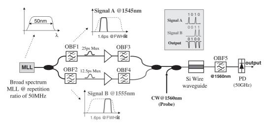
Fig. 12. Silicon based NOR gate—experimental setup.
