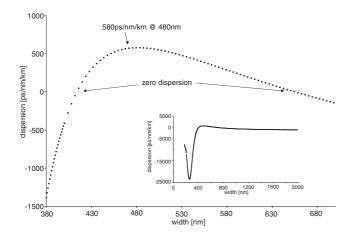
Fig. 2. Dispersion of the TE-like ground mode in a wire with 220 nm Si thickness and oxide cladding.
