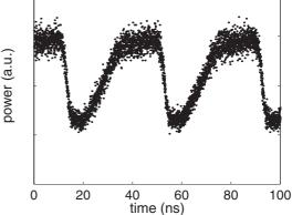
Fig. 17. Measured probe signals at the shorter (a) and the longer (b) wavelength side of the resonance for a peak pump power of 0.66 mW. On the lower wavelength side, the converted data streams corrresponds to 10001000..., while on the other side, 01110111... is obtained.
