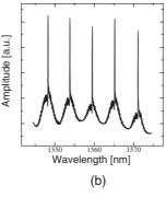
Fig. 11. (a) Time domain trace of modulated CW1 (b) Spectrum of the five modulated CW signals.
