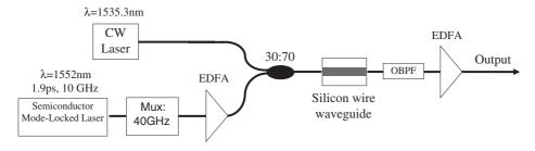
Fig. 8. Ultrafast switching in silicon wire waveguides: simplified experimental setup.
