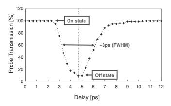
Fig. 10. Pump-probe measurements: response time.
