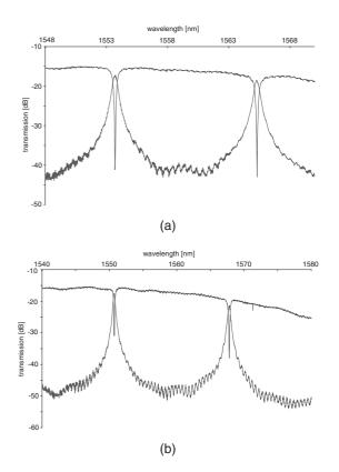
Fig. 7. Fiber-to-fiber transmission spectra of ring resonators with  $5\,\mu m$  radius.
