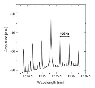
Fig. 9. Optical spectrum of 40 GHz modulated CW signal.
