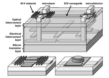
Fig. 1. Top: general layout of an SOI-based optical interconnect on CMOS. Bottom: two possible candidates for the membrane microlaser. Left: DBRmicrolaser. Right: microdisk laser.
