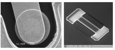
Fig. 2. SEM pictures of a fully processed microdisk laser (top) and an unfinished membrane DBR-microlaser (bottom).
