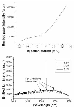
Fig. 3. Measurement results of an electrically injected membrane microdisk laser.
