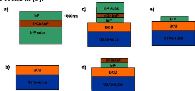
Figure 1 Bonding principle. a) layer-structure. b) host-substrate (e.g. GaAs) with BCB. c) bonding of epi-structure onto the host substrate. d) removing of the InP-substrate. e) removing of the etch-stop layer.
