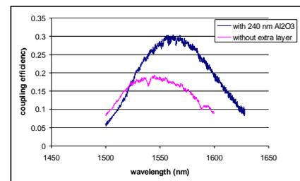
Figure 4 Coupling efficiency of a 1D-"bottom-grating coupler."
