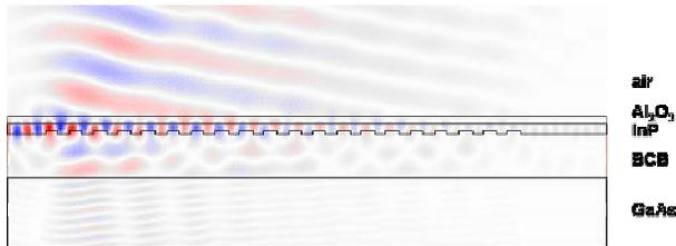
Figure 3 Field profile of a "bottom-grating coupler".
