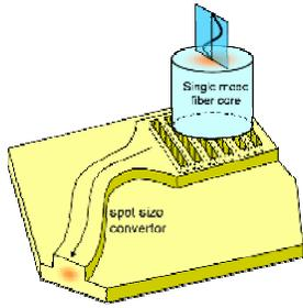
Figure 2 Fiber-to-waveguide coupling by gratings.
