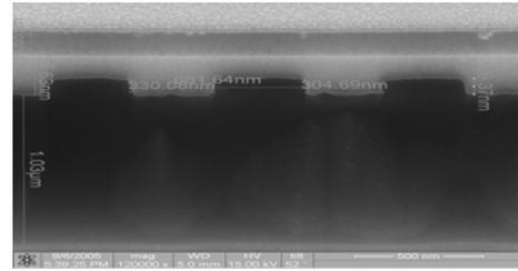
Figure 3 Cross section of a fabricated 1D grating coupler.
