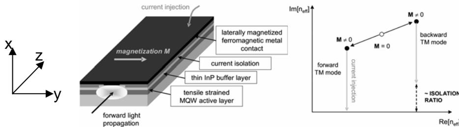
Fig.1 : Schematic representation of the integrated optical isolator and operation principle.
