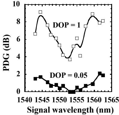
Figure 5 (a): PDG spectrum when pump DOP is 1 and 0.05
