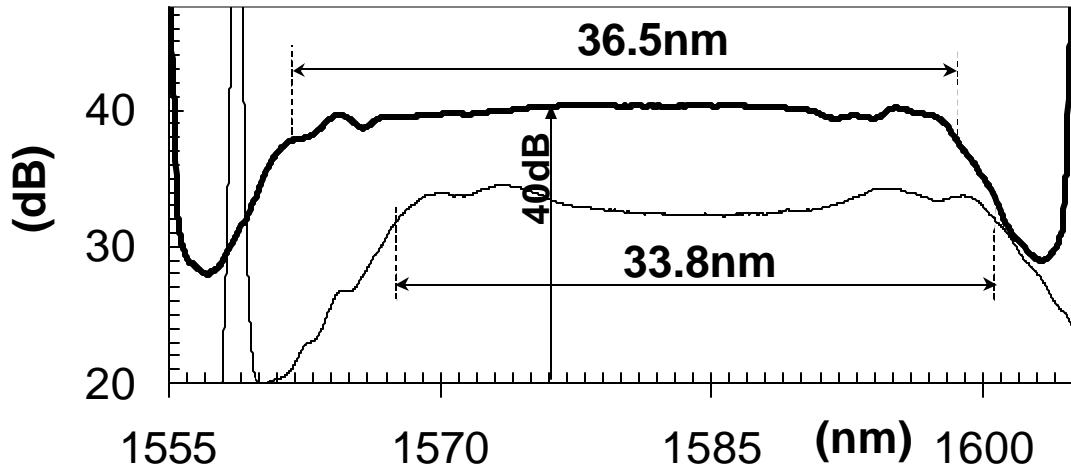
**Figure 2:** CW performance achieved using nearly identical 1km-long HNLF sections. Heavy curve corresponds to HNLF section with  $\lambda_0 = 1578\text{nm}$ , while thin curve indicates HNLF with  $\lambda_0 = 1583.5\text{nm}$ . Latter curve downshifted for 5dB for clarity.
