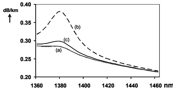
Fig. 3 E-band loss curves: (a) target with 0.285 dB/km loss at 1383nm, (b): example of G.652-c limit loss of 0.38 dB/km at 1383 nm for a fibre specified as 0.38 dB/km @ 1310 nm and (c) current best result from pilot PCVD series
