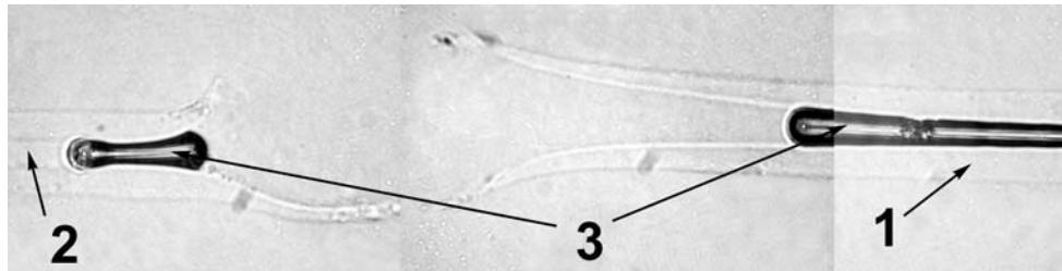
Fig. 3. The etched fiber section disintegrated after the optical discharge stopping. The picture was taken using immersion. Table 1, #8. 1 - silica cladding; 2 – undisturbed fiber core; 3 — bubbles or voids formed in the core after optical discharge passing. The bubble at the left corresponds to the discharge stopping point. The width of the frame is 250  $\mu\text{m}$ . The laser radiation propagated from the left to the right.
