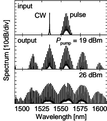
Fig. 2. Optical Spectra of LS-HNLF input and output.  $P_{\text{pump}}$  is input pulse power.
