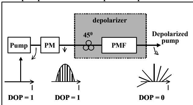
Figure 1 (a): Concept of pump depolarizer using a PC followed by PMF
