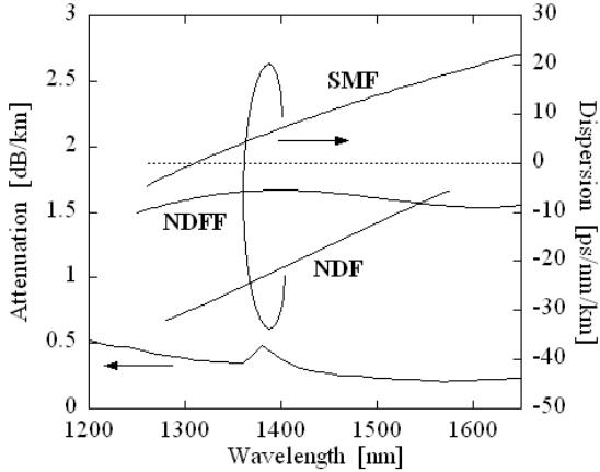
Fig.1 Typical attenuation and dispersion property of fabricated NDFF. Dispersion curves of SMF and NDF are also plotted.
