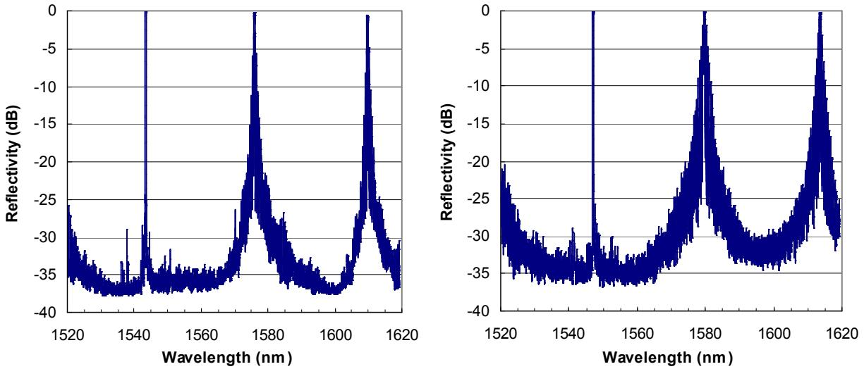
Fig. 3: Extended spectral measurements showing sidebands induced by the phase modulation used for the apodization of a 25 GHz (left) and 50 GHz (right) WDM filter.
