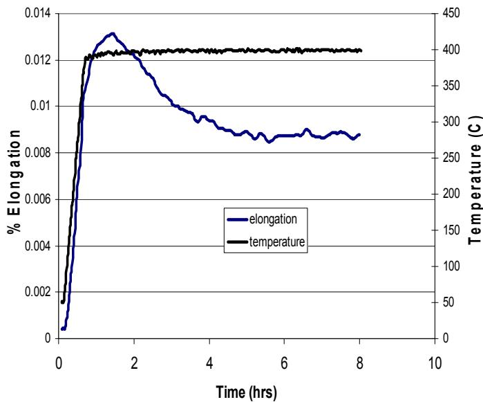
Figure 3. Isothermal relaxation of synthetic silica fiber.
