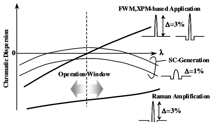
Fig. 1 Schematic chromatic dispersion spectra of HNLFs for various applications
