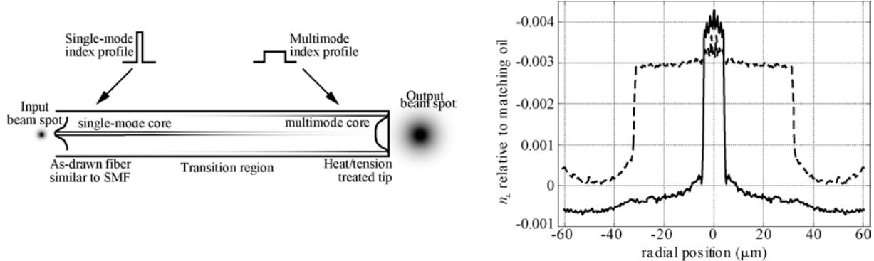
Fig. 2. Schematic illustration of all-fiber beam expanders fabricated with the aid of frozen-in viscoelasticity (left). Refractive index profiles of beam expander fiber: as-drawn (solid line) and after brief heat treatment (dashed line). [13,17]
