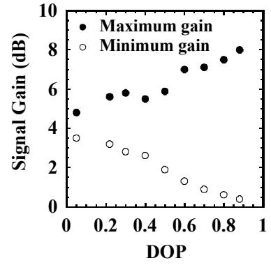
Figure 4 (b): Maximum and minimum signal gain versus DOP of the pump
