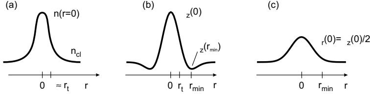
Figure 1. Schematic illustration of a) the refractive-index profile  $n(r)$  versus the radial coordinate  $r$  in the fiber with core radius  $\rho$ , b) the profile of the longitudinal stress component  $\sigma_z(r)$ , c) the profile of the radial stress component  $\sigma_r(r)$ .
