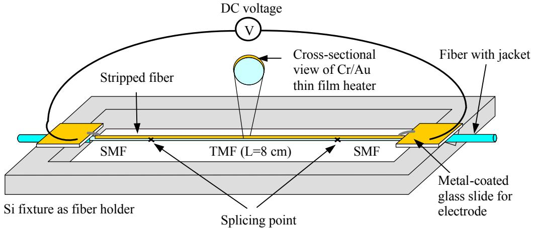
Fig. 2: Schematic of the electrically tuned all-fiber comb filter
