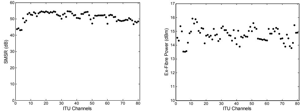
Fig. 5. (a) Side mode suppression ratio (SMSR), (b) Fibre coupled power.
