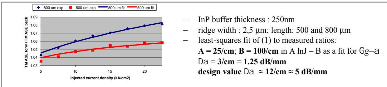
Fig. 4: TM ASE ratio measurements on a 250 nm InP buffer sample (width = 2,5  $\mu$ m)
