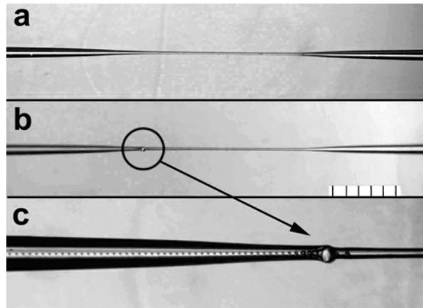
Fig. 1. Waist-formed length of SMF28 (Table 1, #1). **a** – before the optical discharge propagation, **b** and **c** – after the optical discharge propagation. One division of the scale corresponds to 0.1 mm for **a** and **b**; **c** – the width of the frame corresponds to 1 mm. The laser radiation propagated from the right to the left.
