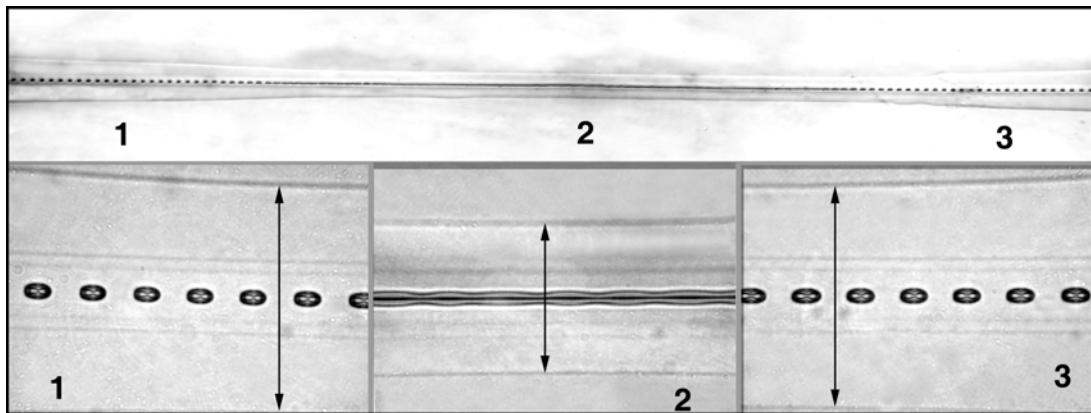
Fig. 2. Waist-formed section of the fiber after the optical discharge propagation without stopping, Table 1, #9. At the top of the figure is the general view of the fiber section, at the bottom regions 1,2 and 3 are shown at an enlarged scale. The laser radiation propagated from the left to the right. Scale: 1—the length of the arrow 64.5  $\mu\text{m}$ ; 2—the length of the arrow is 42  $\mu\text{m}$ ; 3 – 63  $\mu\text{m}$ .
