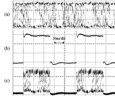
Fig. 3. Timing diagrams for (a) the 10 Gb/s NRZ data signal, (b) the synchronized control signal with pulse duration of 130 ns period, (c) the switched 10 Gb/s data signal at 1553.32 nm. The time scale is 50 ns/div.
