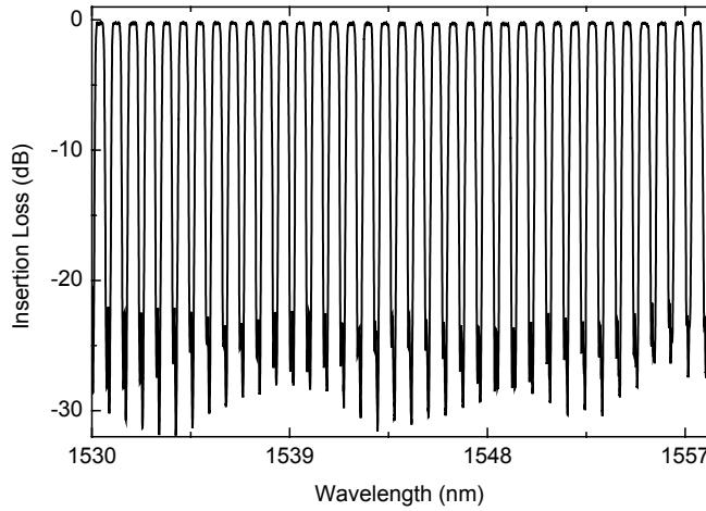
Fig. 1: Transmission spectrum of a single comb filter with 36 channels spacing by 100GHz
