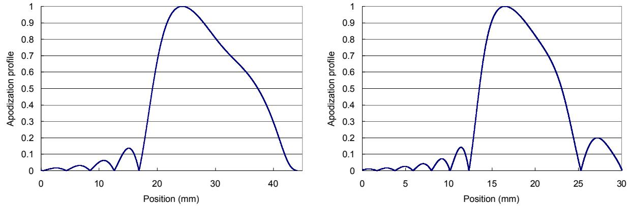
Fig. 1 : Apodization profiles for 25 GHz (left) and 50 GHz (right) low dispersion WDM filters.
