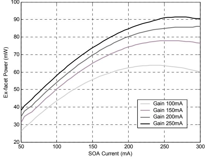
Fig. 2. Ex-facet chip powers in free running mode as a function of SOA current.
