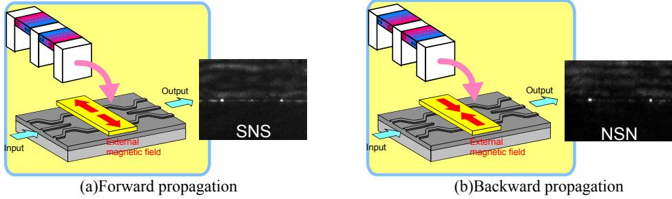
Fig. 3. Measured performance of an optical isolator with a semiconductor guiding layer. Transmittance from the output port is dependent on the magnetization direction.
