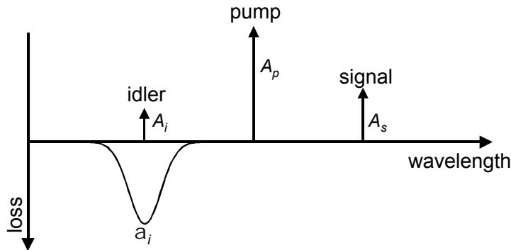
Fig. 1. Single-pump OPA configuration considered in this paper, where the fiber has large distributed loss at the idler wavelength.
