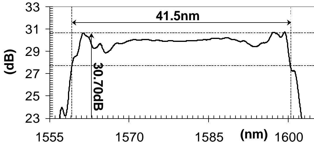
Figure 1: Equalized (3-dB bandwidth) parametric gain using 500m-long HNLF section and two-pump PA design.
