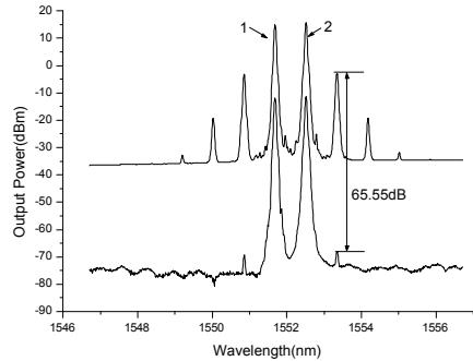
Fig. 2. The output spectra of the FWM signals with (top curve) and without (bottom curve) the Raman pump. The Raman power for the top curve is 1.1 W. The input data signal and the control signal are labeled ‘1’ and ‘2’, respectively.
