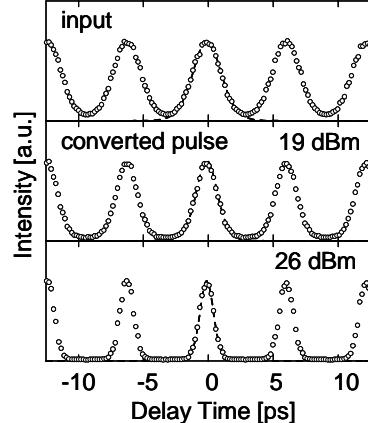
Fig. 3. Autocorrelation traces of input and converted pulse trains. Number in upper right indicates input pulse power  $P_{\text{pump}}$ . Dashed lines are Gaussian shapes.
