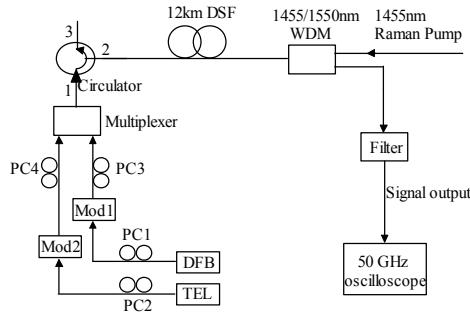
Fig. 1. The experimental setup of Raman-assisted FWM.
