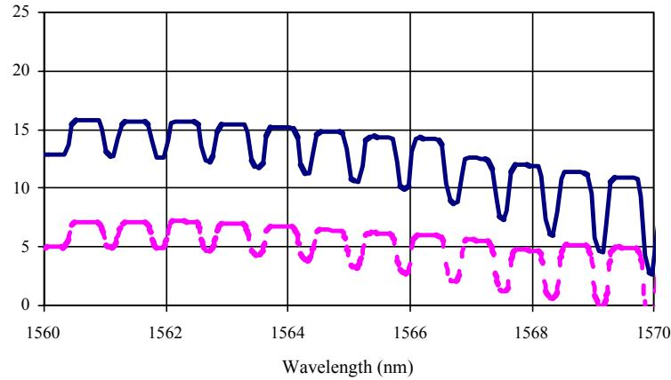
Fig. 2. OPA gain spectra for: identical (solid line) and orthogonal (dashed line) pump SOPs in randomly-birefringent fiber.
