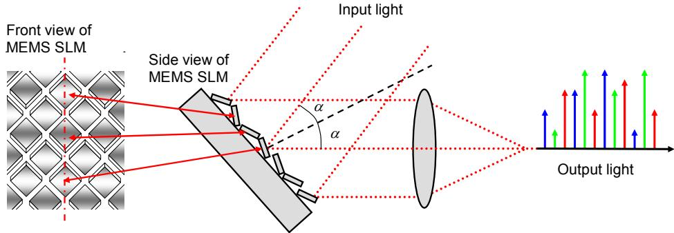
Figure 2. Implementation of interference based MEMS filter using commercial MEMS SLMs. The input light is normal to the SLM surface, and only the parts of the input that illuminate micromirrors that are rotated to the right interfere to create the output. Each row of the SLM corresponds to a certain time delay or height, and the height distribution required to create a desired filter is therefore created by rotating to the right the correct number of mirrors in each row.
