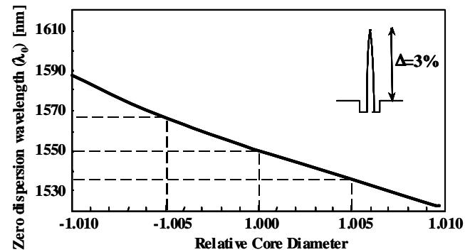
Fig. 2 Calculated relationship between zero dispersion wavelength and core diameter
