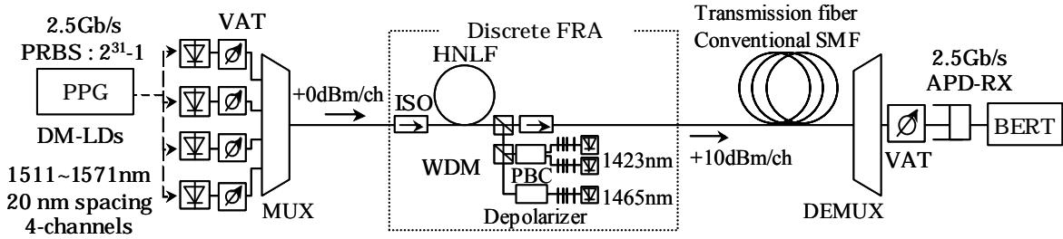
Fig.4 Experimental setup of fiber Raman amplifier for 4-channels CWDM systems
