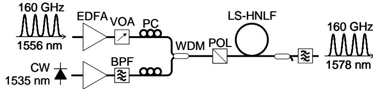
Fig. 1. Experimental setup of wavelength conversion of 160 GHz ps pulse train.
