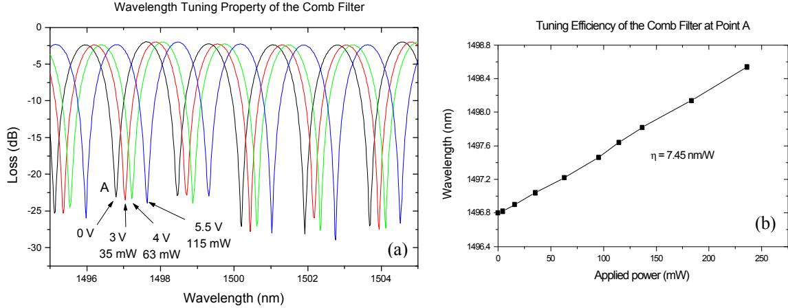
Fig. 3: (a) Wavelength tuning of the comb filter with a thin film micro-heater, (b) Tuning efficiency of the comb filter.
