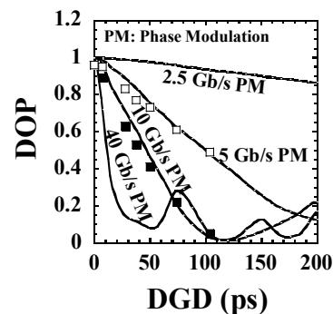
Figure 1 (b): Performance of the depolarizer under different phase modulation speed. Simulation: solid lines; experimental: squares
