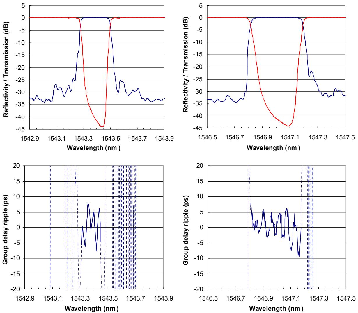
Fig. 2: Top: Measured reflectivity/transmission spectra for the 25 GHz (left) and 50 GHz (right) WDM filters.
