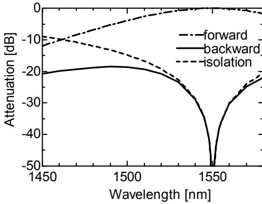
Fig. 2. Calculated wavelength dependence of the interferometric isolator. The wavelength dependence of material properties is taken into account.
