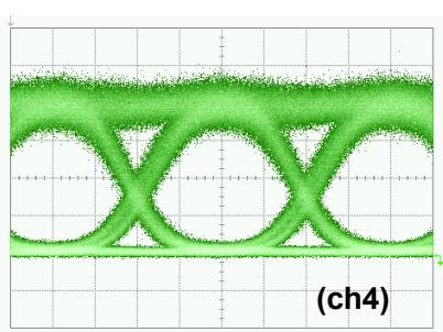
Figure 5. Typical eye diagram for 12.5-Gbit/s operation.
