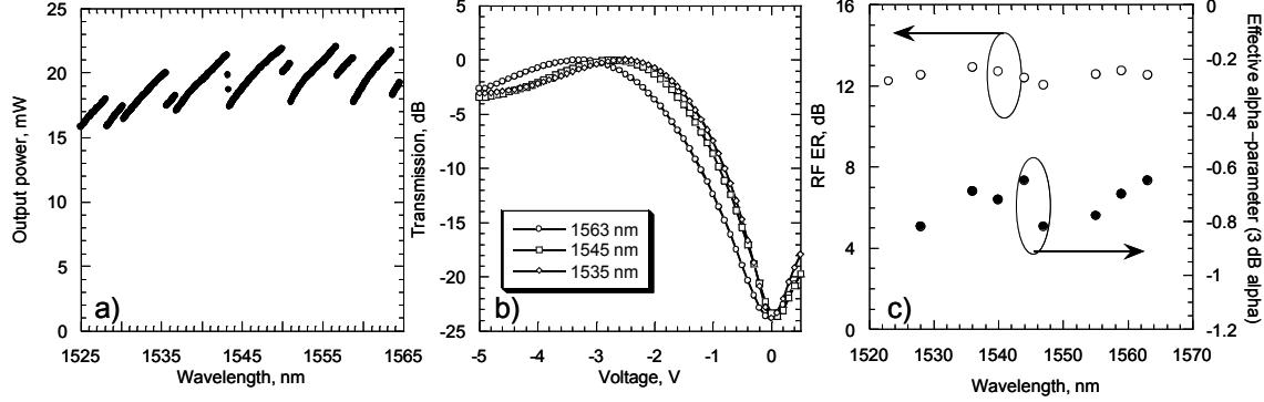
Fig. 2. a) Unleveled SG-DBR-SOA-MZM output power across the tuning range. b) Normalized transmission characteristic for three wavelengths. c) RF ER and 3 dB alpha parameter in single-ended drive configuration across the tuning range.
