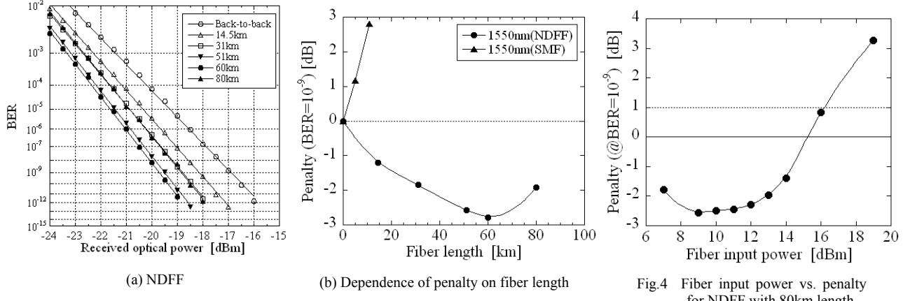
Fig.3 Measured transmission performance for  $1.55\mu\text{m}$  signals.
