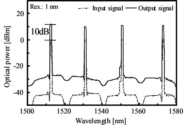
Fig. 5 CWDM signals observed at the input and the output of FRA
