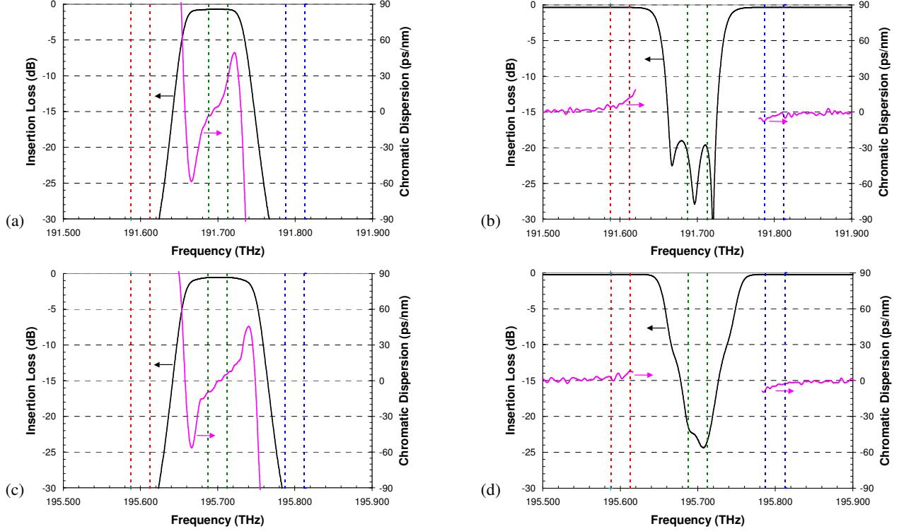
Fig. 1. (a) Measured transmission amplitude and CD of a packaged 100 GHz thin film bandpass filter with square passband; (b) Measured reflection amplitude and CD for square passband filter; (c) Measured transmission amplitude and CD of a packaged 100 GHz thin film bandpass filter developed for low CD; (d) Measured reflection amplitude and CD for low CD filter. Vertical dotted lines represent 25 GHz passbands for three adjacent channels.
