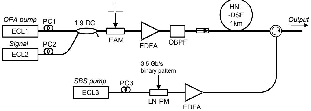
Fig. 2. Experimental setup to demonstrate the loss-induced OPA. PC: polarization controller, OBPF: optical bandpass filter, LN-PM: LiNbO<sub>3</sub> phase modulator
