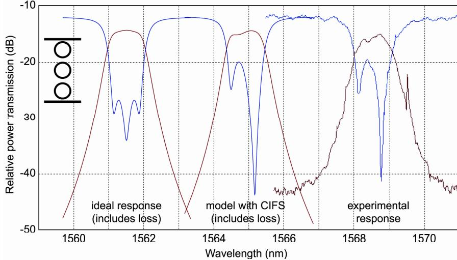
Fig. 2. Drop and thru port frequency responses of a 3rd-order filter using identical microrings (inset diagram): ideal theoretical response (left plot); theoretical model incorporating the expected net CIFS in the middle ring of +20GHz from CMT (middle plot); experimental measurement of the response of fabricated filter based on three identical rings (right plot). Loss is fit into the models to match experiment. Theoretical spectra are displaced horizontally for clarity in the plot.
