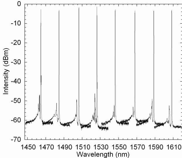
Fig. 4. Superimposed VCSEL emission spectra from the WDM VCSEL array measured at a constant absorbed pump power of 14 mW at 20 °C.
