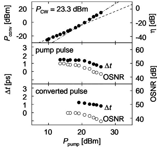
Fig. 4. Converted pulse power  $P_{\text{conv}}$  v.s. input pump pulse power  $P_{\text{pump}}$ , and dependence of temporal duration  $\Delta t$  and OSNR of converted pulse train on  $P_{\text{pump}}$ .  $\eta$  is conversion efficiency.  $P_{\text{CW}}$  is assisted CW power. Dashed line and dotted-dashed line in upper part indicate square and cubic, respectively.
