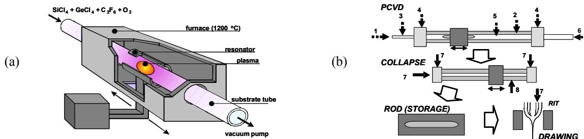
Fig. 1 Setup of a PCVD core production machine (a) and total process flow (b) with arrows showing potential sources of contamination
