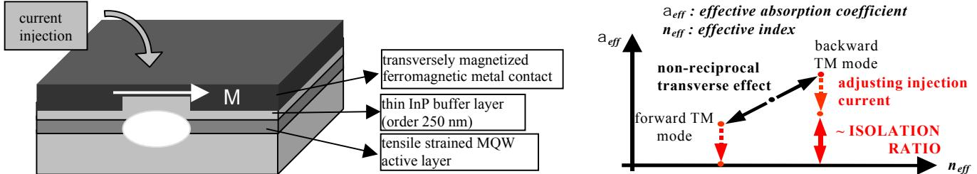
Fig. 1: Schematic of the operation principle of the proposed isolator
