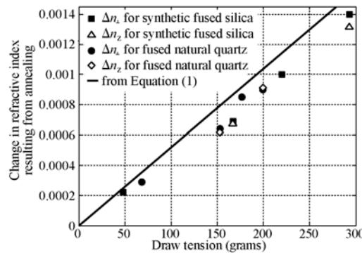
Fig. 1. Annealing-induced index change measured in a 125  $\mu\text{m}$  diameter fiber compared to Eq. (1).
