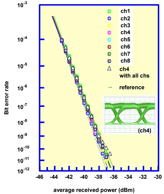
Figure 4. BER performance and typical eye diagram (inset)
