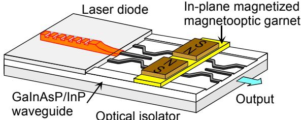
Fig. 1. Schematic drawing of an optical isolator integrated with a semiconductor laser
