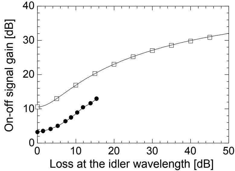
Fig. 3. On-off signal gain measured as a function of the idler loss (dots). The results of analytical calculation (Eq. (3)) (solid line) and the split-step Fourier simulation (squares) are also shown.
