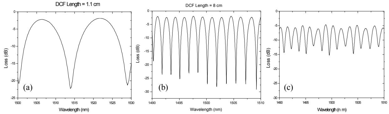
Fig. 1: (a) and (b) Filtering spectra of the comb filter with different TMF lengths; (c) Filter response when a non-optimized shorter arc time is used.
