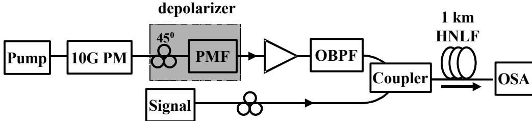
Figure 2: Experimental setup. PM: phase modulation, OBPF: optical bandpass filter, HNLF: highly nonlinear fiber
