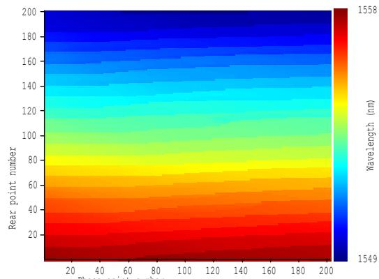
Fig. 4. An example of a rear-phase tuning plane.
