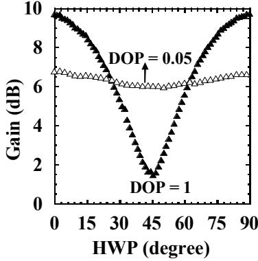
Figure 3: Signal power gain changes against SOP of input signal when DOP is 1 and 0.05
