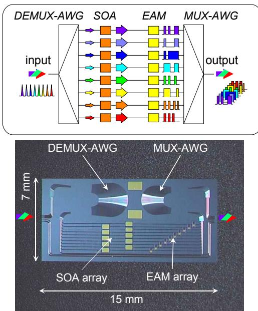
Figure 1. Functional diagram (top) and photo of the chip (bottom).
