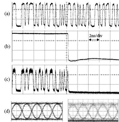
Fig. 4. (a) – (c) Same as Figure 3 but the time scale is 2 ns/div, (d) eye diagrams of the input data signal (left) and switched data signal at 1553.32 nm (right). The time scale is 50 ps/div.
