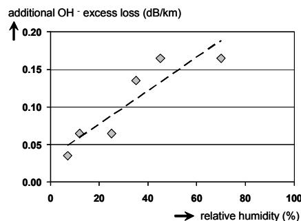
Fig. 2 Effect of reduction of relative humidity on OH<sup>-</sup> excess loss compared with an arbitrary reference level.
