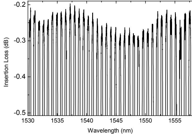
Fig. 2: Detail show of the top of the transmission spectrum in Fig. 1. The variation channel to channel is less than  $\pm 0.1\text{dB}$
