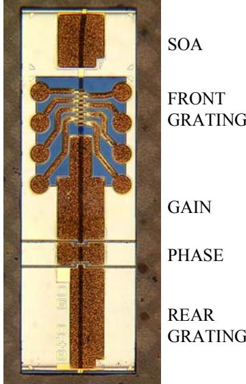
Fig. 1. DS-DBR laser chip.
