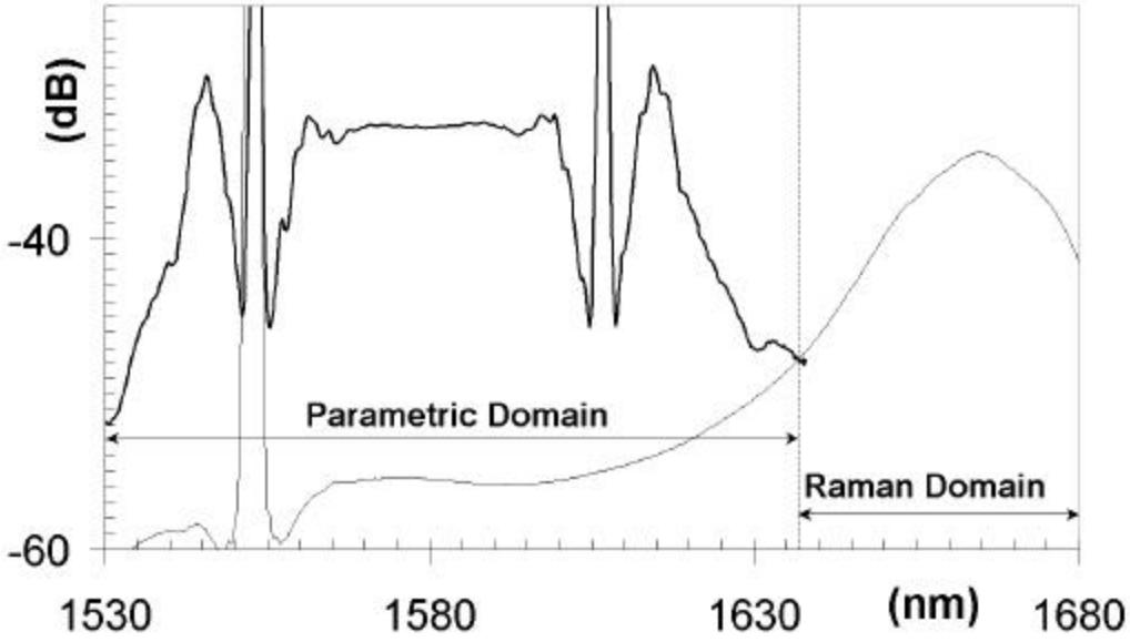
**Figure 3:** Domains of significant parametric (heavy curve) and Raman (thin curve) are well separated.
