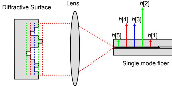
Fig. 1. Schematic drawing of diffractive optical filter.
