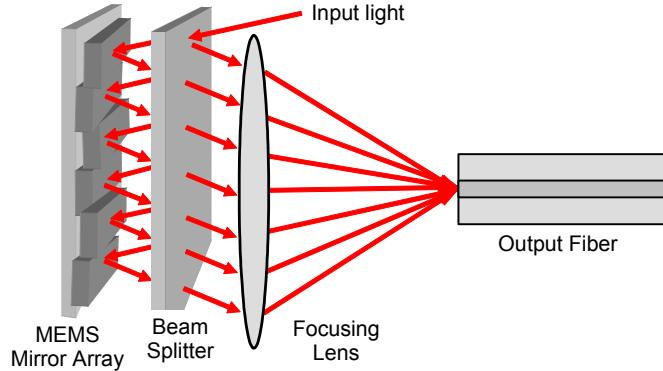
Figure 3. Schematic structure of the MEMS Gires-Tournois interferometer/filter. The phase shifts controlled by the micromirrors determine the transfer function of the filter.
