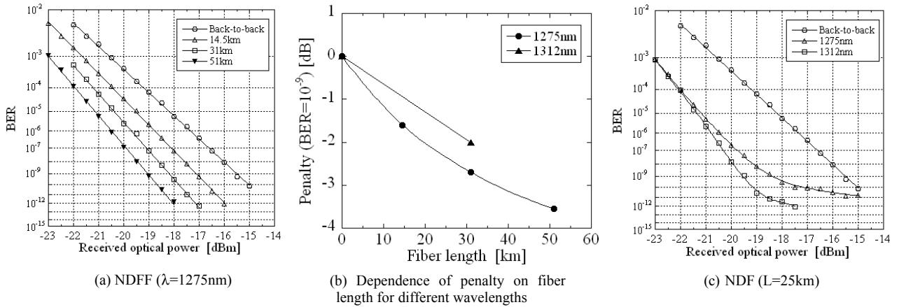
Fig.2 Measured BER data for 1.3 $\mu\text{m}$  band signals.
