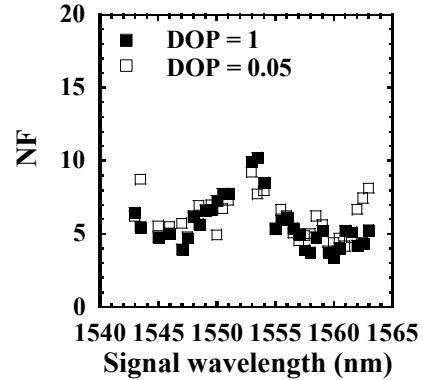
Figure 5 (b): NF of the amplifier before and after pump depolarization
