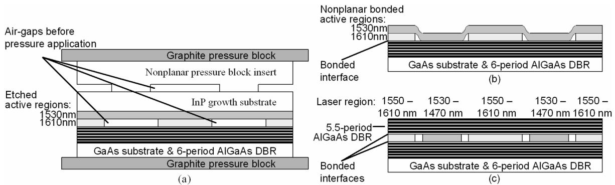
Fig. 1. Process-flow cross-section schematic of a wafer section showing: (a) nonplanar pressure block against back of step-etched InP active region wafer in bonding fixture, (b) VCSEL active regions bonded to AlGaAs DBR with InP growth substrate removed, (c) complete VCSEL array structure after bonding second AlGaAs DBR and removing GaAs substrate.
