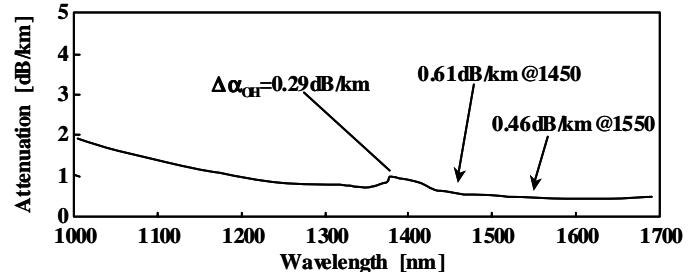
Fig. 3 Attenuation spectrum of the HNLF for Raman Amplification
