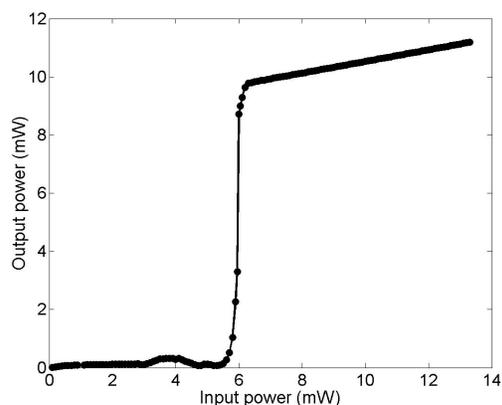
Figure 2: Experimental obtained transfer characteristic of the 2R regenerator described in [5] based on a MZI with a GCSOA in each arm.
