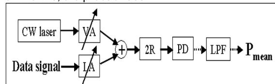
Figure 1: Illustration of the used configuration. VA: variable attenuator, LA: linear amplifier, 2R: a 2R regenerator, PD: photodiode and LPF: low pass filter.
