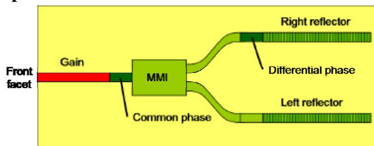
Figure 1. Schematic drawing of the Modulated Grating Y laser
