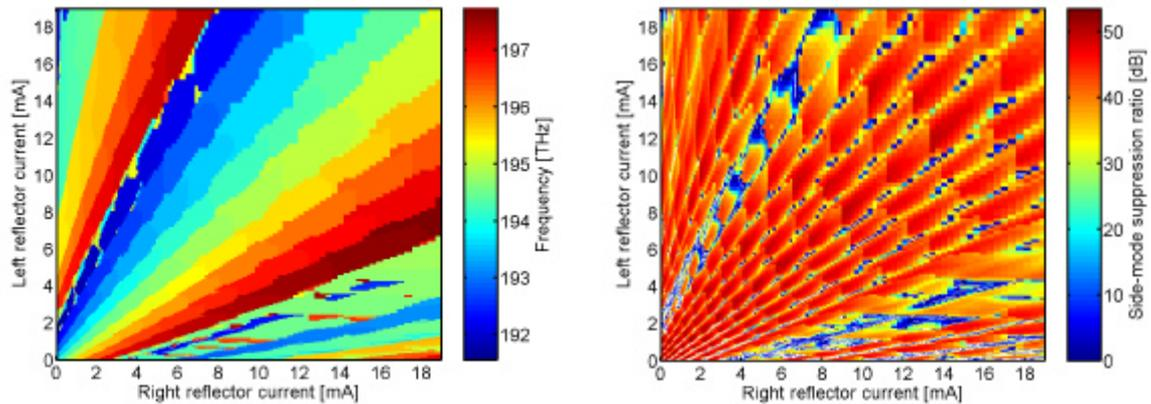
**Figure 3. Measured contour maps of the frequency and the side mode suppression in function of the two reflector currents**
