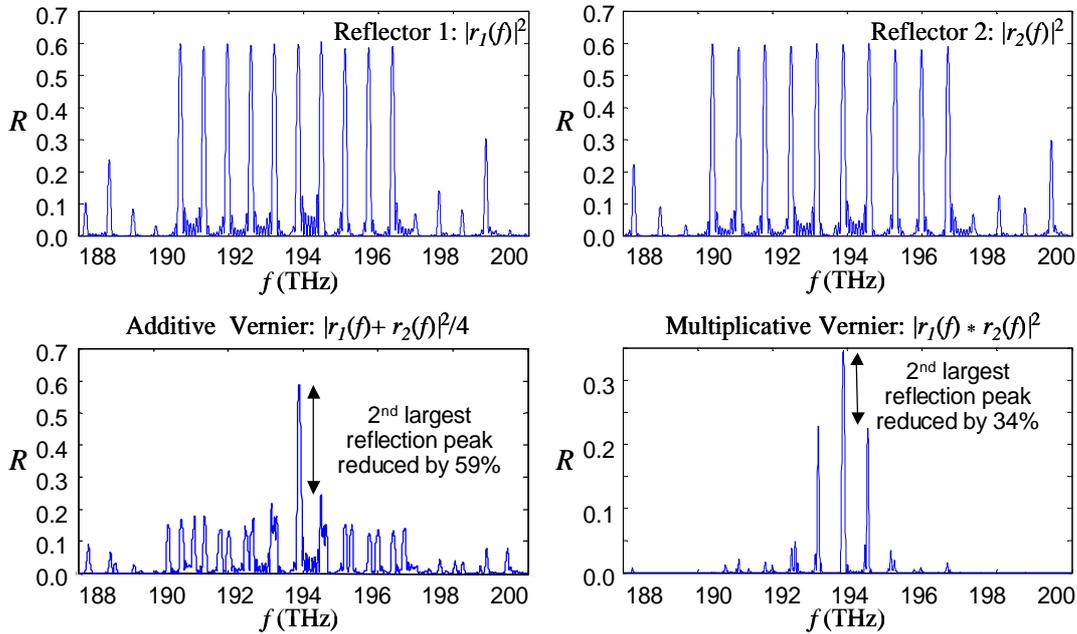
**Figure 2. Reflection Spectra of the two reflectors (top figures) and the comparison between the additive (MGY) and multiplicative (SSG-DBR) Vernier effect (bottom figures)**
