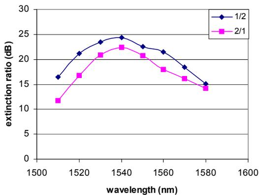
Figure 4a. Extinction ratio measurement
