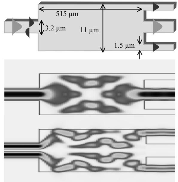
Figure 3a: Mode splitter dimensions
