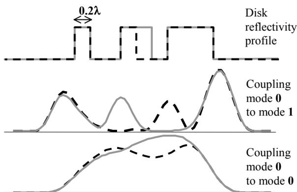
Figure 2a: Two bit pattern with bit length  $0.2\lambda$
