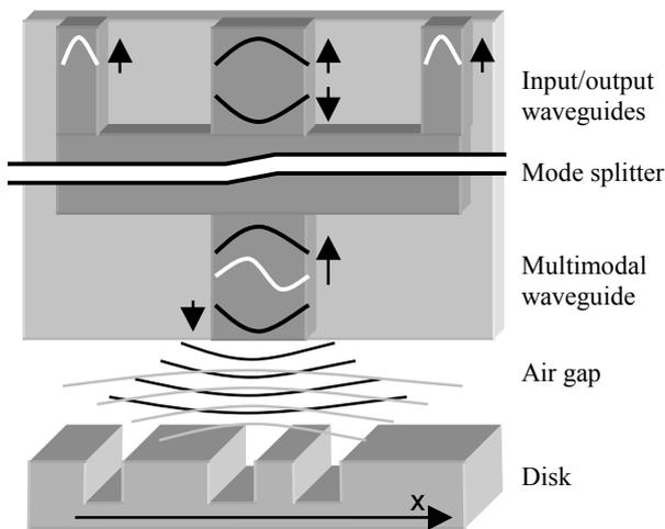
Figure 1: Schematic view of the PIC, waveguide and disk.
